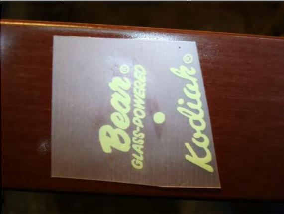
You can see in this pic of where I rubbed the transfers into the tacky finish better. I use a razor blade to pick up the edge of the transfer paper.
