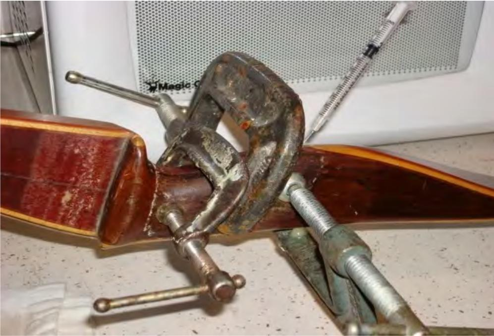
This is the 3rd syringe full it took to fill the I-beam. That's OK better then not getting any into the crack. But make sure the crack is filled and kind of flooding over a little.
