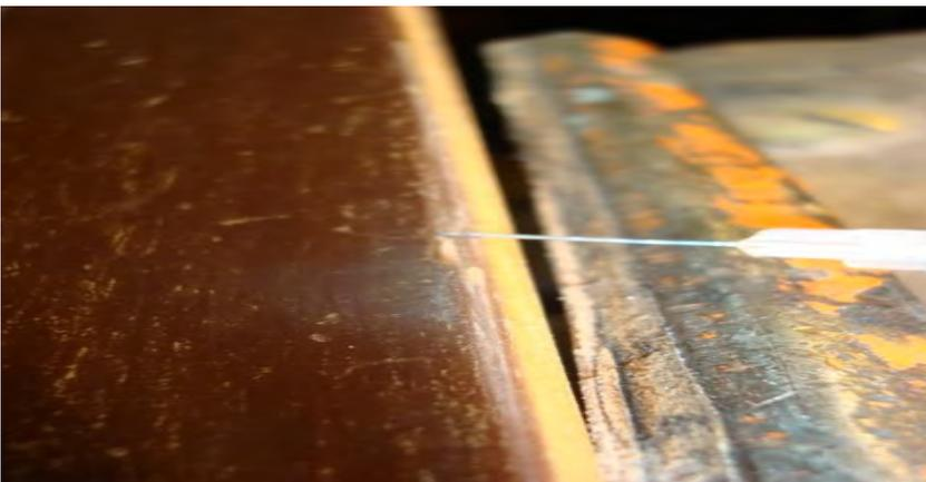
See those? Bear Archery would tell you to break those off with a pair of needle nose pliers so they do not snag on anything and paint over that spot with some clear finger nail polish. I like to glue them down and wait 24 hours and then pick at them with the needle of the syringe. If any are not glued down, I normally try and sand them out when ever possible.
