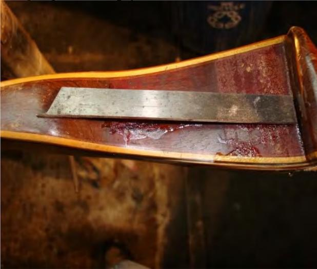
Once you have either used a small scraper or sand paper and removed all the dry glue. Most of the old finish will get scraped or sanded off as well. Check and see if the gap is filled. If not get a pick or small nail and remove all the uncured glue. Then fill it again.
