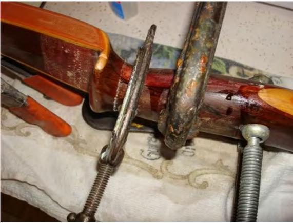
Add 2-3 more clamps wherever you can, Good idea to stay as near the crack as possible. 5 clamps with about 2-3 pounds of pressure each. Now wait about 12-24 hours until the LT gets inside the crack which is not getting exposed to the air so much will have plenty of time to dry
