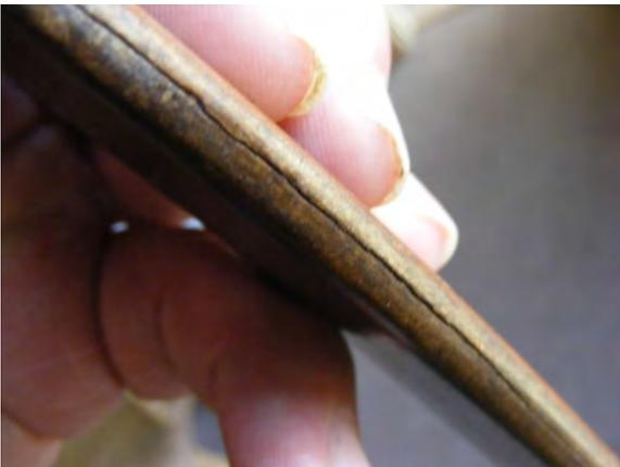
Here are a few more pics of tip overlay repair for Shawn. The 60" 1957 Kodiak Special has factory wood & paper tip overlays. I had to replace one and used wood & black fiberglass to make the repair. The red canvas micarta in the pic will be to make underlays for the 66" KS. It has a tiny bit of fiberglass damage on the belly side right near the string grooves.
