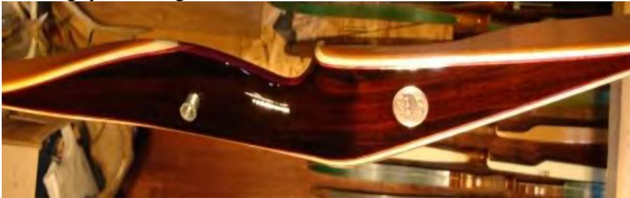
The best way to remove the grip is just peel it open at the seam and peel it off however you can. Sometimes they are a little stubborn and you will have to actually scrap the old leather off. I use a small wood scraper on lots and lots of leather grips.
