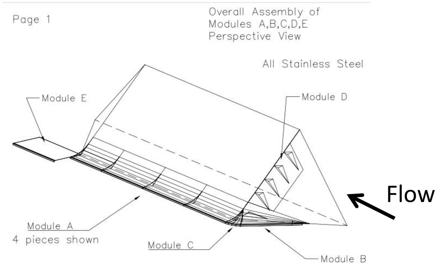
**Example stainless steel scAUR™ retrofit for a spill-through abutment.**
