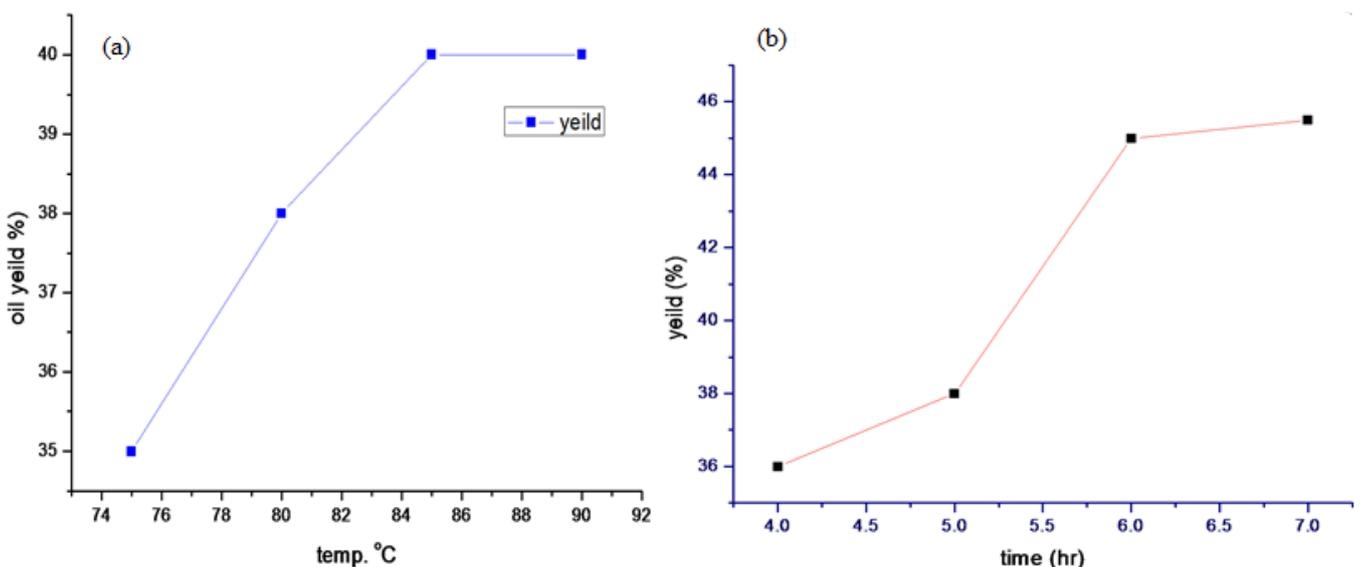
Fig.6. (a) Timperature and (b) time influences of oil yeild during oil extraction from blended algae with sludge
