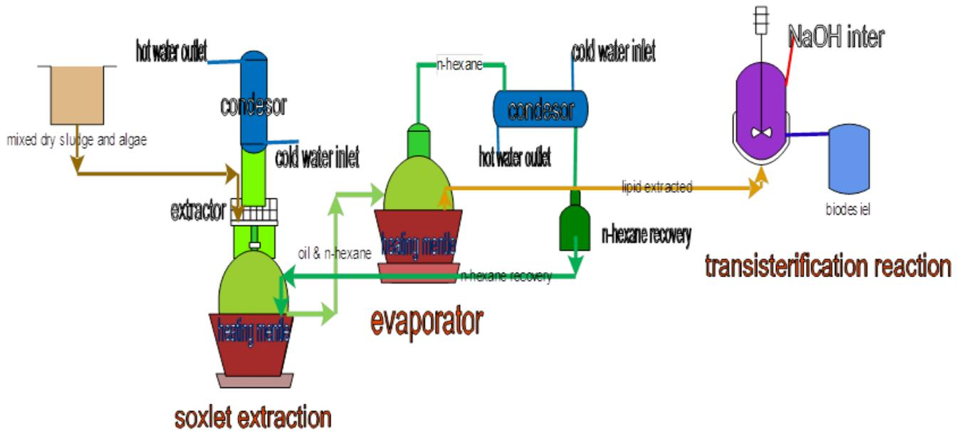
Fig. 3. Overall lipid extraction and biodiesel production from waste for sustainable development
