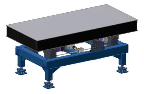
This DLS two degrees of freedom High Precision Motorized Optical Table used Newport Corporation Research Grade breadboards with a grid of M6 tapped holes. The system base was made of a welded steel frame with a powder coated finish. Frames were filled with sand to reduce the table natural frequency and provide passive damping. When in use, the table rests on four machinery feet. When in transport, the feet are retracted and casters allow for easy handling.
