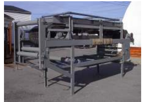
Remanufactured vacuum belt filter with all new components and a special, epoxy coated frame.
