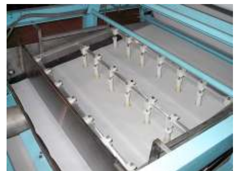
Rebuilt plow section and TriStar Filter Belt
