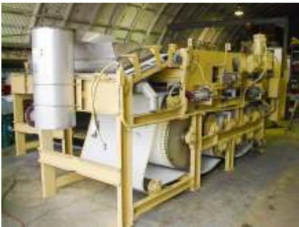
Remanufactured three-belt design belt filter with new TriStar belt. Frame was completely stripped, treated, and electrostatically painted.
