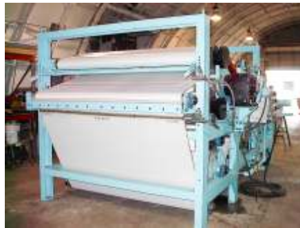
Fully restored belt press for municipal sludge dewatering features newly painted frame, new TriStar belt, and all new controls.
