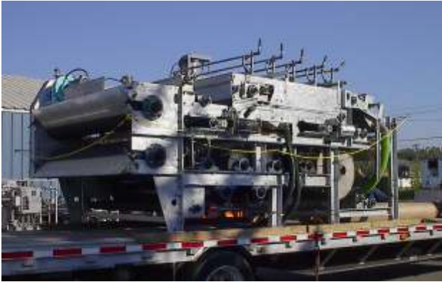
Remanufactured belt filter by TriStar LTD. Completely rebuilt including sand-blasted & galvanized frame, resurfaced rollers, new bearings, new steering controls, and conversion from pneumatic to hydraulic control.
