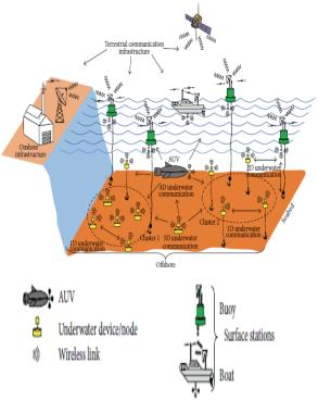
Fig.1: Underwater sensor network architecture [6] However, UWSN applications are exciting but challenging at the same time. The reason lies in unpredictable conditions of water environment which creates serious constraints in the design and deployment of such networks. The focus of this paper is to survey the available UWSN application. The paper further focuses on classifying these applications and presenting a summary for each class.
