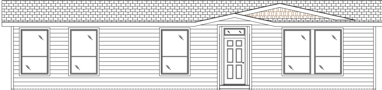
FRONT SIDEWALL W/NOMINAL 24'-0" EYEBROW DORMER
