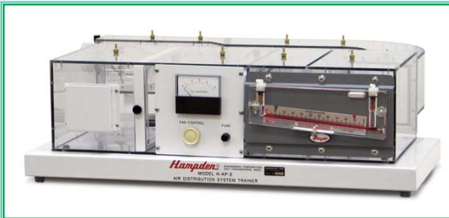
The Hampden **Model H-AP-2** Air Distribution System Trainer is designed to acquaint the student with the fundamentals of air movement found in typical forced air heating and air conditioning systems. The trainer aids the student in acquiring a better understanding of static pressures, velocity pressures, and air volumes. The trainer shows the student how air moves under various conditions created in the distribution system.
