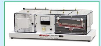
The Hampden **Model H-AP-2** Air Distribution System Trainer is designed to acquaint the student with the fundamentals of air movement found in typical forced air heating and air conditioning systems. The trainer aids the student in acquiring a better understanding of static pressures, velocity pressures, and air volumes. The trainer shows the student how air moves under various conditions created in the distribution system.
