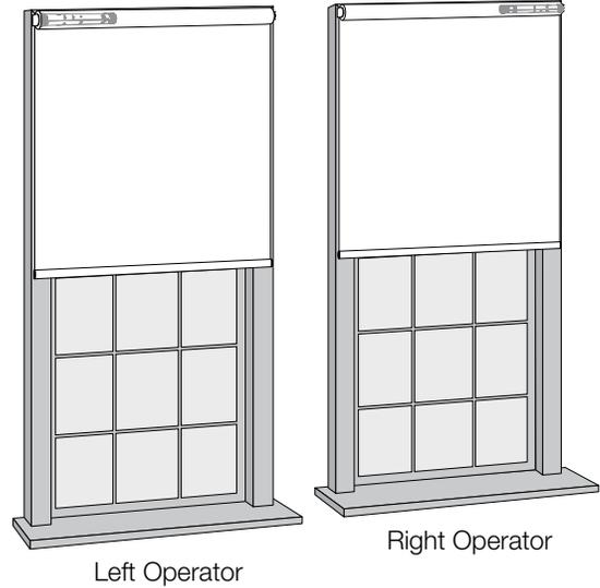
In some installations, operator side choice may be related to battery access clearance. Please refer to **Battery Access Clearance**, later in this document.
