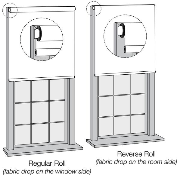
**NOTE:** Reverse roll is recommended for dual-sided fabric, otherwise the shade roll will be a different color than the hanging fabric.
