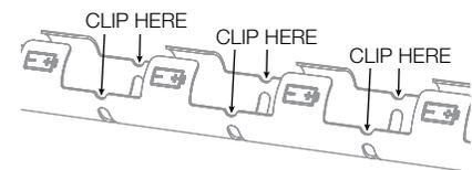
2. *Battery sleeve clearance is less than 3 in (76 mm), and/or bracket mounting depth disallows battery access:* Extend the Operator bracket, then press the shade release to remove the shade from the brackets for battery installation or removal.
