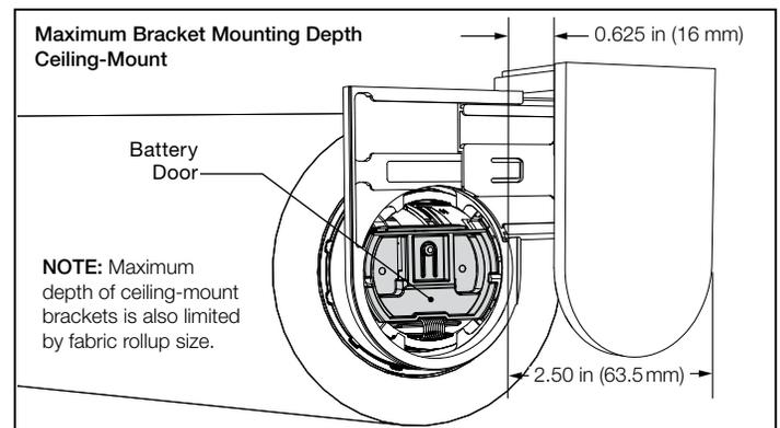
**Battery Sleeve Removal/Insertion:** Batteries are housed in a sleeve that fits inside the EDU. Removal and insertion of the sleeve requires clearance to end walls and other window-adjacent objects or structures.\*
