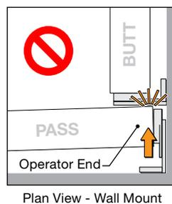
**IMPORTANT:** Plan to allow at least 1/4 in (6 mm) clearance between the pass shade fabric roll and the butt shade bracket. This is required because there is some movement at the idler end of the fabric roll when the operator bracket slide ring is extended. The exact amount of clearance needed to prevent fabric-bracket contact varies with shade size.
