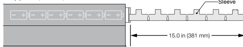
\* **Close-quarters Installations:** When the installation location does not allow the battery access shown above and/or battery sleeve clearances shown at left, the following methods may be used.
