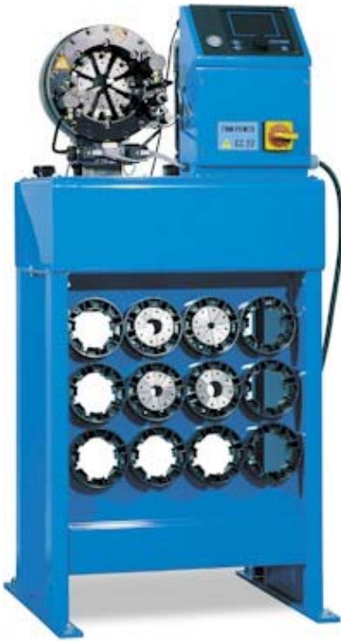
Finnpower CC22-IS 68 ton up to 1-1/4" hose, high-speed capability
