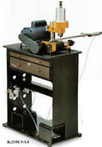
Rabbit K250USA4-1P Handles 3/8" to 2-1/2" tube diameter. Cuts 1" 0.095 wall carbon in 1 second
