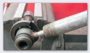
Position the new gear on the shaft, replace the stop nut, and then stake to re-upset the side of the drive shaft into the stop nut holes to lock the nut.
