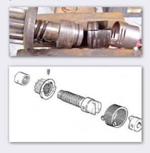
Pry away the old sleeve and clean the end of the Bendix shaft at the groove, then slip on the new sleeve. The sleeve has two slits. The center portion between the slits is carefully folded down with a tool into the shaft groove. Some early shafts use a forward groove, so fold down the slit there. The sleeve will be secure but still allow the sleeve to spin. Don't clamp the slit portion too much; turn the sleeve with your fingers and it should rotate without binding.
