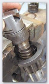
If the drive gear needs to be replaced, the stop nut at the end of the screw shaft must be removed. It is right-hand threaded onto the screw shaft and locked by the two tiny holes on the outside of the stop nut which are crimped on the inside of the shaft. Use a small punch and clear the upset crimp on drive shaft inside the stop nut and unscrew to remove.
