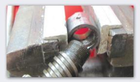
Finally, confirm that the small drift pin and spring in the drive gear edge contacts the threaded shaft. This little, but important, pin and spring provides the resistance needed to keep the drive gear from accidentally drifting into the ring gear while the engine is running.
