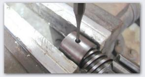
A longer bolt threaded into the shaft provides leverage for a pipe or other tool to turn the shaft counter-clockwise while the stop nut is held fast in the soft jaws of a vice.
