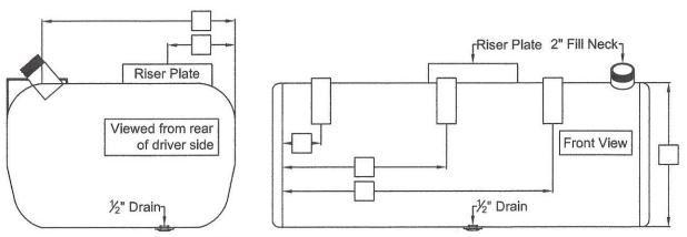
Please note: All sizes are NPTF unless otherwise noted and reference all measurements from the lateral weld seam and the end cap weld seam to the center of the fittings.
