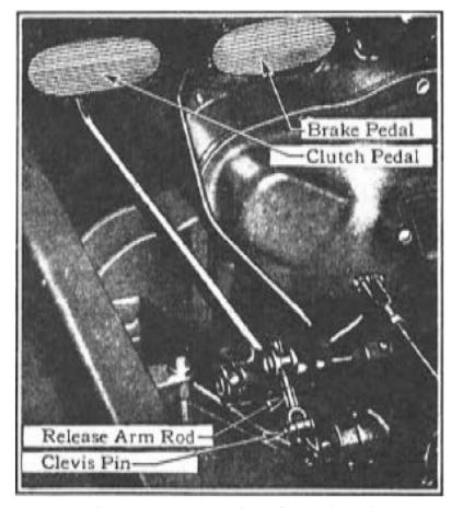
decreases the clutch pedal play. Screwing the rod *out* increases the play. After making the adjustment, be sure to replace the clevis pin and cotter key.
