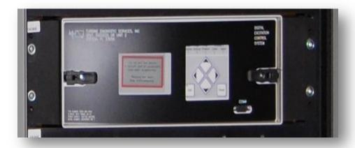
The 400 Series Digital Excitation Control System is a microprocessor based controller that provides excitation control, flexible logic control and optional power plant system stabilization for synchronous machines in an integrated package. These are most often incorporated in upgrades for SCT/PPT, potential source SCR bridges, Amplidyne, ALTERREX, GENERREX and the larger brushless and rotating DC exciters.
