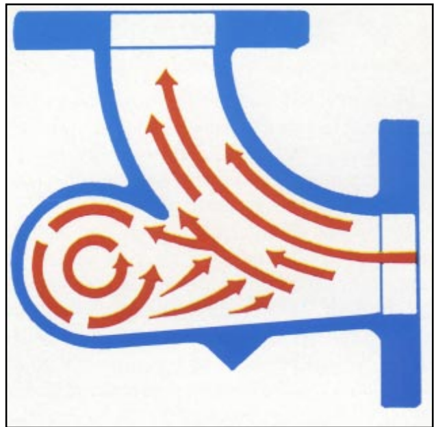
Cross section of a Smart Elbow™. The ball of material in the pocket slowly rotates and deflects incoming material smoothly around the corner, virtually eliminating wear, turbulence, and pressure drop.
