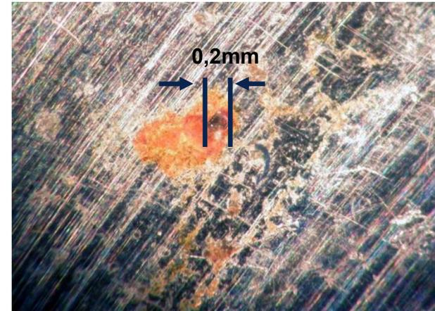
*Destruction of the diaphragm via pitting corrosion*
