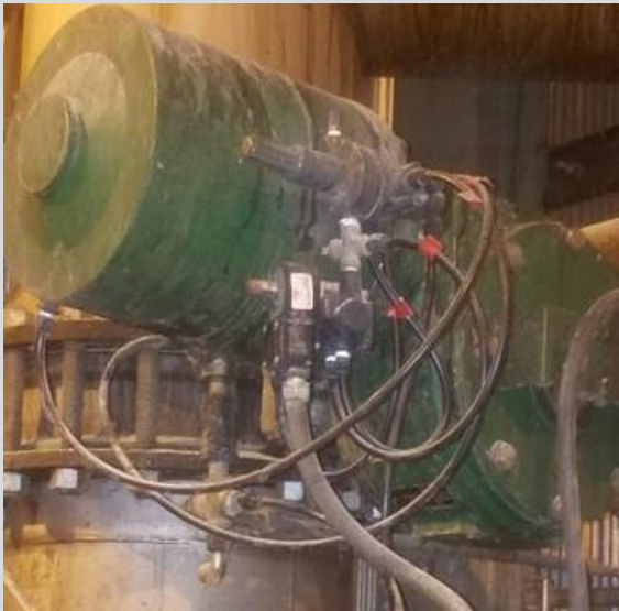
Complex ad-hoc piping and integration with various components to achieve fail-safe with external air reservoir.
