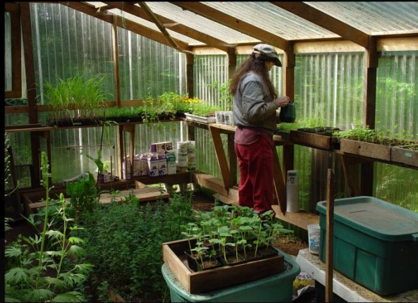
Greenhouse Located In Clearing Between House And Watershed (looking east) 16 feet by 20 feet; Lexan Throughout. Base 4 x 6 Raised Off The Ground On Cement Blocks.. Cross Ventilation Heated Wood Or Propane The Lexan Sheet Was Run Down To Ground Level Outside Greenhouse Is Located A Rabbit Hutch Which, At The Time Of The Was Home To An English Angora. Greenhouse Was Provided With A Gardener
