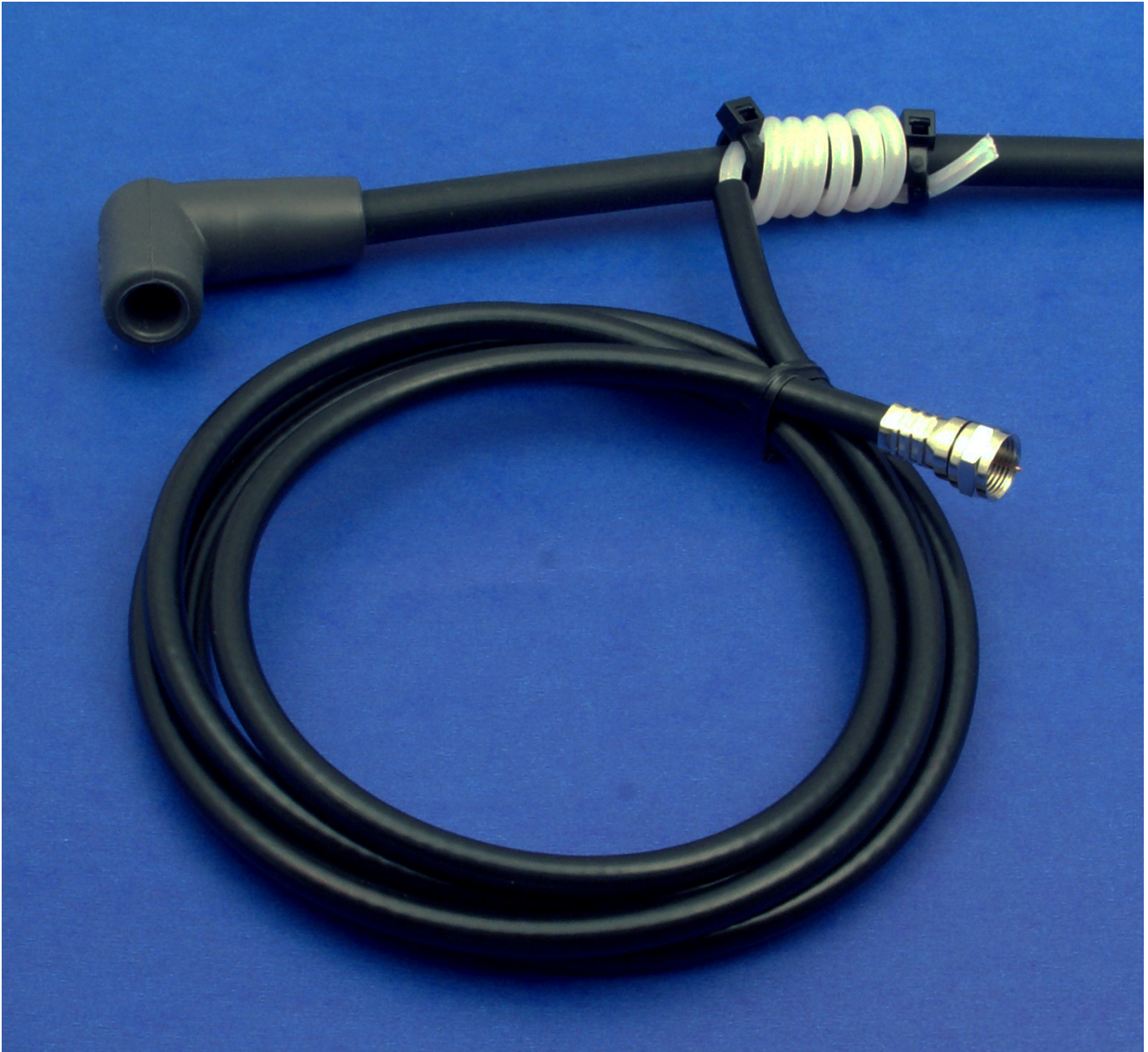
Figure 5 – Capacitive Spark Pickup on Spark Plug Wire
