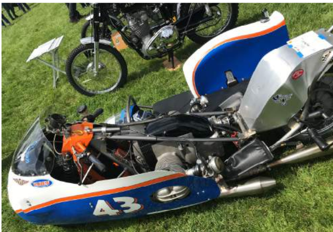
Class P2 sidecar racing rig. Has custom frame, pre-1972 engine, 336 sport cam, dual ignition, 5 speed transmission.
