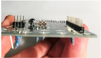
Insert JP1 and JP2 onto the front (silk screen side) of the PCB. Solder one pin at either end. Double check the header is on a right angle and is flush with the PCB. When you are happy, solder the rest of the pins.
