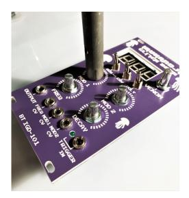
Place washers and nuts onto the 4 pots. Tighten the nuts, again using a tube spanner or ring spanner to avoid scratching the front panel.
