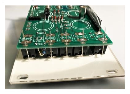
Unscrew the 10mm stand-off located in the upper corner of the PCB. Insert the 1mm nylon washer onto the screw and replace the 10mm stand-off on top of the washer.
