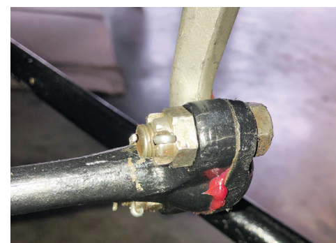
Nuts secured to bolts and cotter pins placed, and locked.
