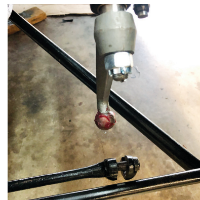
Steering ball or pitman arm fitted on steering shaft and greased.
