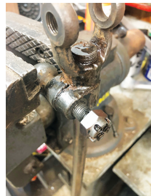
Removing nut from yoke ball
