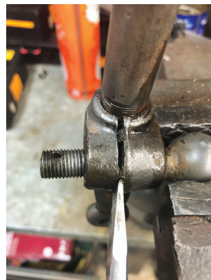
Spreading of yoke split with chisel
