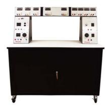
The Hampden **Model HMD-100-CM-DA-CDL** Mobile Console provides the facilities required to perform experiments with Series 100 Motors and Generators plus power and metering services. The Student Experimentation Station allows experiment values and test results to be directly fed into typical PC data acquisition boards (not included), such as Data Translations, Analog Devices and Metrabyte.
