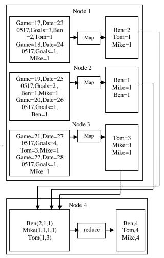
Fig.6: Example of Program Flow
