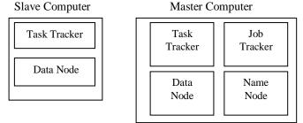
Fig.3: Components of Master and Slave Computers
