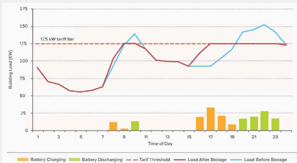
Figure 2 – Use of Energy Storage to Reduce Peak Demands
