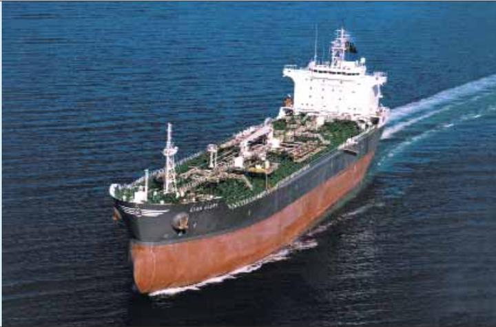
Single screw diesel engine driven Oil Product / Chemical Tanker with longitudinal bulkhead, bulbous bow, and transom stern. Living quarters including navigation bridge, engine room with fuel oil tanks on both sides and pump room located aft. Double bottom / double side tanks and peak tanks intended for segregated ballast. Cargo space divided into sixteen (16) cargo and two (2) slop tanks. Hull structure made of mild steel. Eight (8) grades of cargo can be handled simultaneously.
