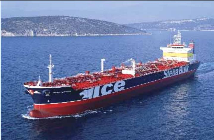
Single screw diesel engine driven Oil Product Tanker with longitudinal bulkhead, bulbous bow, and transom stern. Living quarters including navigation bridge, engine room with fuel oil tanks on both sides located aft. Double bottom / double side tanks and peak tanks intended for segregated ballast. Cargo space divided into twelve (12) cargo, two (2) slop tanks and residual tank (1). Hull structure made of mild and higher tensile steel. Six (6) parcels of cargo can be handled simultaneously.
