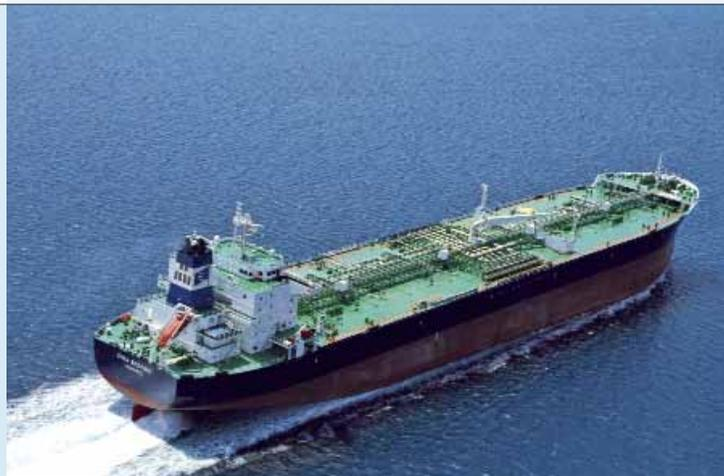
Single screw diesel engine driven Oil Product Tanker with longitudinal bulkhead, bulbous bow, and transom stern. Living quarters including navigation bridge, engine room with fuel oil tanks on both sides and pump room located aft. Double bottom / double side tanks and peak tanks intended for segregated ballast. Cargo space divided into twelve (12) cargo and two (2) slop tanks. Hull structure made of mild and higher tensile steel. Six (6) grades of cargo can be handled simultaneously.
