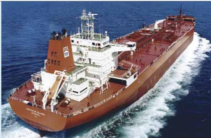
Single screw diesel engine driven Oil Tanker with longitudinal bulkhead, bulbous bow, and transom stern. Living quarters including navigation bridge, engine room with fuel oil tanks on both sides and pump room located aft. Double bottom / double side tanks and peak tanks intended for segregated ballast. Cargo space divided into twelve (12) cargo and two (2) slop tanks. Hull structure made of mild and higher tensile steel. Four (4) grades of cargo can be handled simultaneously.
