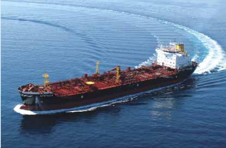
The vessel is double hull tanker for oil and oil products and IMO type 2 tanker for chemicals. Cargo space is divided into seven pairs of cargo tanks, one pair of slop tanks and one retention tank. The structure of cargo tanks is designed for cargo density of 1,025 t/m<sup>3</sup> in completely filled tanks and for cargo density up to 1.55 t/m<sup>3</sup> in partially filled tanks with filling height corresponding to the density ratio, including zig-zag and alternate loading.
