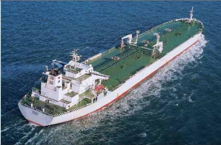
Single screw diesel engine driven Oil Tanker with longitudinal bulkhead, bulbous bow, and transom stern. Living quarters including navigation bridge, engine room with fuel oil tanks on both sides and pump room located aft. Double bottom / double side tanks and peak tanks intended for segregated ballast. Cargo space divided into twelve (12) cargo and two (2) slop tanks. Hull structure made of mild and higher tensile steel. Three (3) grades of cargo can be handled simultaneously.
