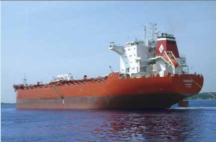
The vessel is suitable for transporting crude oil and dirty petroleum products and chemicals world wide. 18 submerged pumps are fitted in cargo tanks plus two in slop and one in residual tank. One cargo manifold is arranged for two cargo pumps, nine segregations. All cargo tanks are composed of vertical corrugated bulkheads and plane surfaces. Hull structure mild steel.
