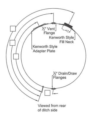
Please note: All sizes are NPTF unless otherwise noted and reference all measurements from the lateral weld seam and the end cap weld seam to the center of the fittings.
