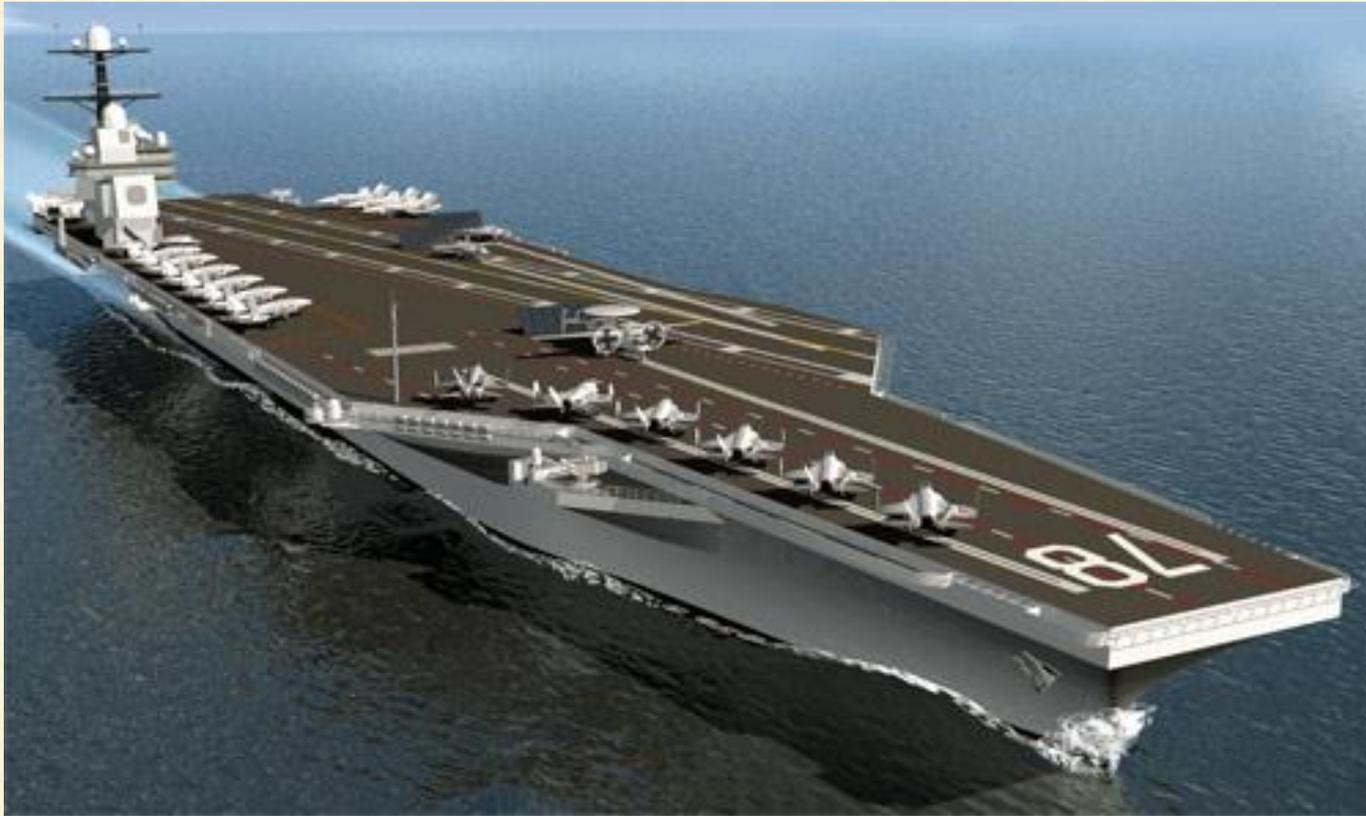
The shape of the hull ensures 97,000 tons of water is displaced while the water level on the outside of the hull is well below any dangerous line
