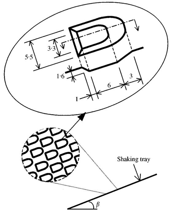
*Fig. 2. Size, shape and arrangement of indents on the surface of shaking tray;  $\beta$ , longitudinal slope angle; all dimensions in mm*
