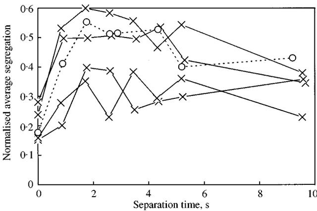
Fig. 5. Comparison of change in segregation condition with separation time between experimental and simulated results using normalized average segregation, which indicates the position normal to the separation plate for paddy relative to brown rice: X, experiment; O, simulation
