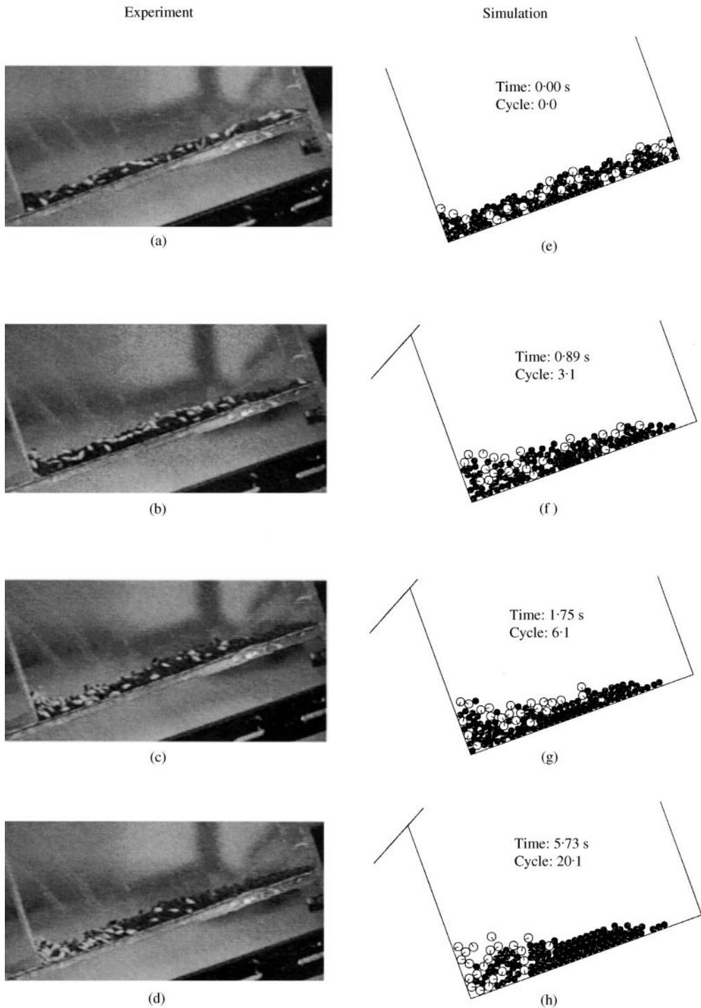
Fig. 4. Snapshots of change in separation condition during separation, where each experimental snapshot (a)–(d) on the left has almost the same separation time as the simulations (e)–(h) shown on the right; white particles indicate paddy rice; black particles indicate brown rice
