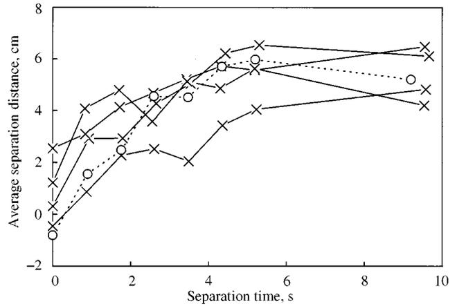
Fig. 6. Comparison of change in separation condition with separation time between experimental and simulated results using average separation distance, which indicates the distance parallel to the separation plate between paddy and brown rice: X, experiment; O, simulation
