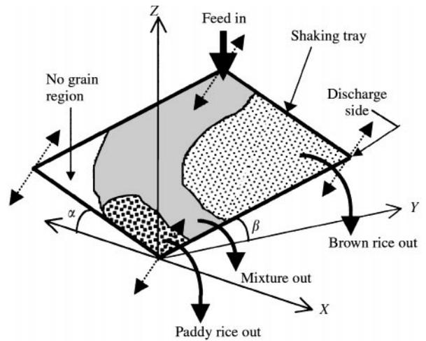
*Fig. 1. Separation condition of grains on shaking tray in an actual system;  $\longleftrightarrow$ , the direction of the tray's oscillation in Y-Z plane; the cross slope angle  $\alpha$  is fixed at  $8^\circ$ ; longitudinal distribution of grains can be controlled by varying the longitudinal slope angle  $\beta$  and the feed rate of the mixture*
