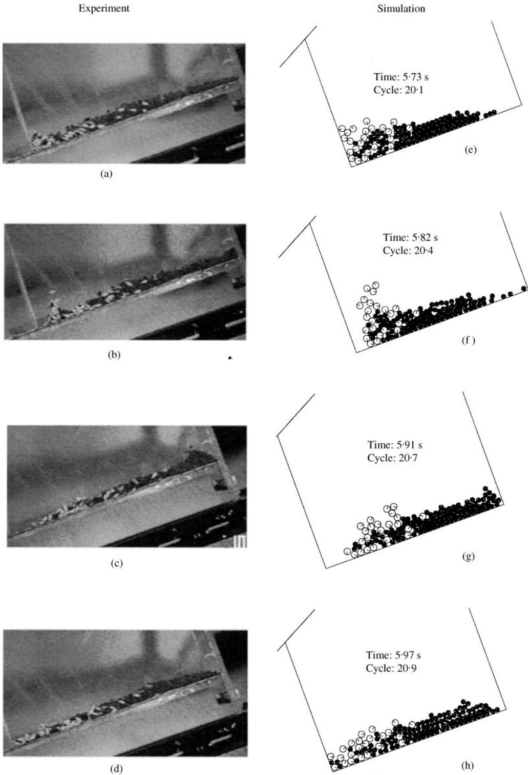
Fig. 3. Snapshots of shaking behaviour of the grain assembly, where each experimental snapshot (a)–(d) on the left has almost the same separation time as the simulations (e)–(h) shown on the right; white particles indicate paddy rice; black particles indicate brown rice
