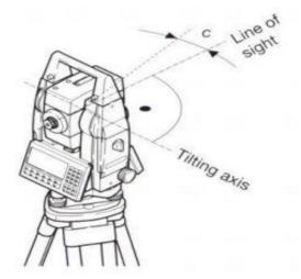
**Vertical axis error (tilting axis error)** errors occur when the titling axis of the total station is not perpendicular to its vertical axis. This has no effect on sightings taken when the telescope is horizontal, but introduces errors into horizontal circle readings when the telescope is tilted, especially for steep sightings. As with horizontal collimation error, this error is eliminated by two face measurements.
