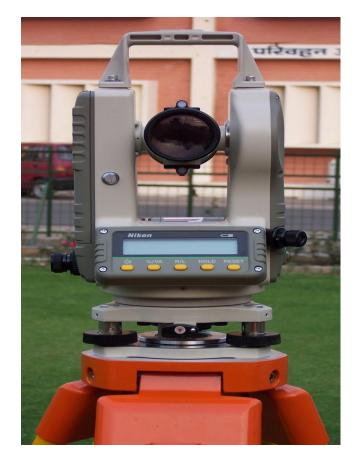
(iii) **Total Station -** This is an electronic instrument. In this instrument, all the parameters required to be observed during surveying can be obtained. The value of observation gets displayed in a viewing panel. The precision of this type of instrument varies in the order of 0.1" to 10".
