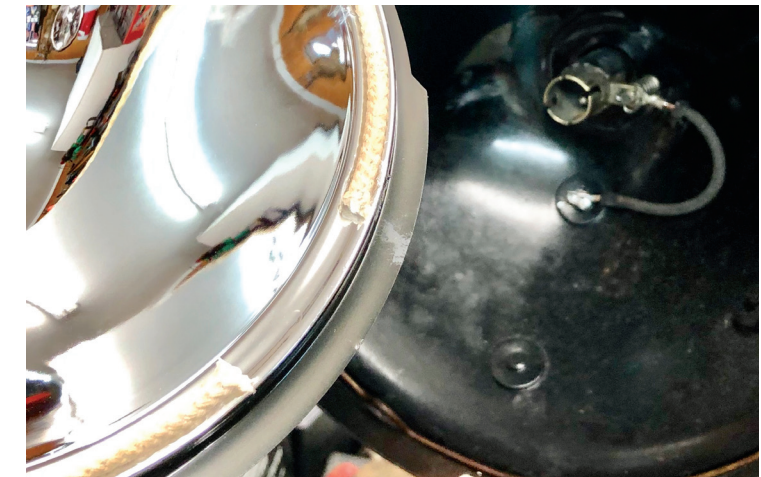
4) Bulb now burns brightly! 5) Headlamp bucket with added ground wire, and a new reflector with highly reflective vacuum metalized aluminum finish for best illumination.
