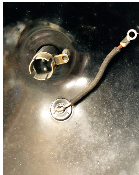
2) Jumper ground wire with ring terminal mounts behind the socket lug over the adjusting screw; the other end is soldered to a rivet.
