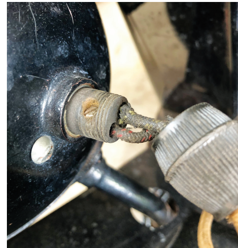
1) Adjusting screw for pulling in or pushing out the bulb socket. (Note the shiny steel rim of the socket in the rear of the headlamp bucket.)
