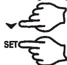
1. Enter the Programming mode by pressing the Set and DOWN key for 3s (LED 1 and \* start blinking).
