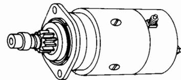
Causes of troubles are often not necessarily in the starter itself nor in the battery, switches, cables, cable connections and defective electrical connections of vehicle grounding
