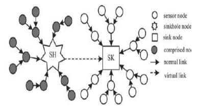
Fig. 1.2: Sinkhole Attack
