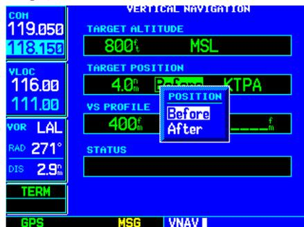
STEP 6: Rotate the **small right knob** to select whether the distance is "Before" or "After" the reference waypoint.
