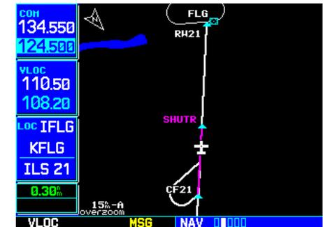
“VLOC” must appear in the lower right corner (above the **CDI** key) in order to use the VLOC receiver with your external CDI and autopilot.
