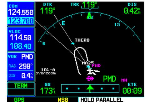
STEP 6: An alert message recommends the holding pattern entry procedure (e.g., "HOLD PARALLEL").
