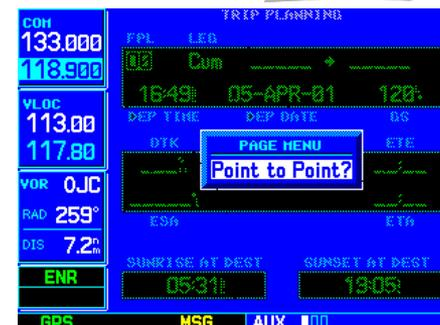
STEP 2: Press **MENU** and use the options window to select the other leg mode: Point-to-Point or Flight Plan.
