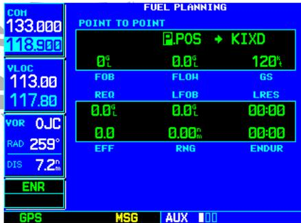
STEP 3a: For direct-to fuel planning, press **CLR** (with the “from” waypoint field highlighted) to display “PPOS” (which represents your present position).
