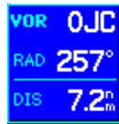
Directly below the VLOC Tuning Window is a VLOC Ident Window (default setting). When the GNS 530 is tuned to a nearby VOR, the VLOC Ident Window displays the Morse code identifier of the selected station, the radial from the VOR and the distance from the VOR. When tuned to a nearby localizer, the VLOC Ident window displays the identifier, associated airport and runway. The VLOC Ident Window can be replaced with traffic information or configurable data fields, as outlined on page 153.
