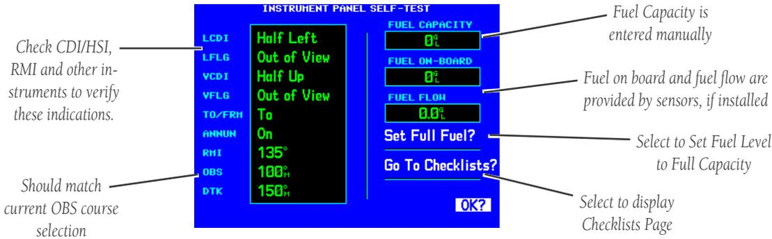
Once the database has been acknowledged, the Instrument Panel Self-Test Page appears. To ensure that your GNS 530 and any connected instruments are working properly, check for the following indications on your CDI/HSI, RMI, external annunciators and other connected instruments:
