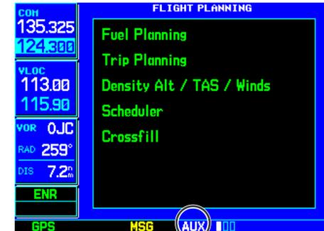
...then, rotate the **large right knob** to select the AUX page group, as indicated by "AUX" at the bottom of the screen. Rotate the **small right knob** to select the desired page within the group.
