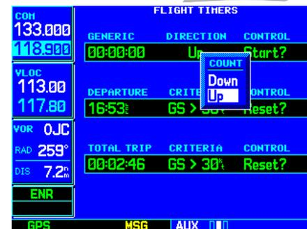
STEP 3 (top): Rotate the **small right knob** to select a count "Down" or count "Up" timer.
