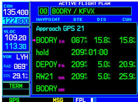
STEP 6: Once you “Activate?” the approach, the Active Flight Plan Page appears showing the sequence of waypoints in the approach.
