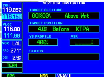
STEP 3 & 4: Rotate the **small** and **large right knobs** to select a target altitude. The target altitude can be above field elevation (for an airport) or you can specify an MSL altitude for any waypoint category.
