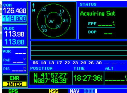
When the GNS 530 is first powered on, an “Acquiring” status appears at the top of the page and no signal strength bars are displayed.
