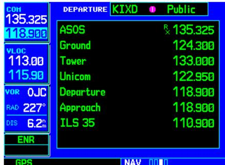
Once the standby frequency is selected, use the **COM flip-flop** key to make the frequency active for transmit and receive operations.
