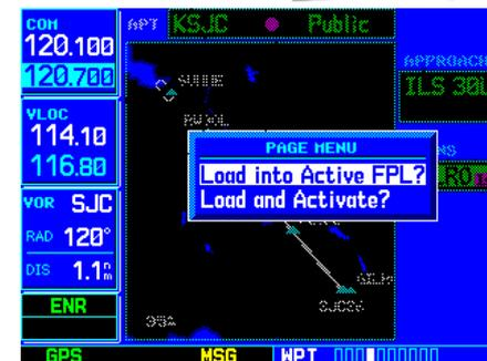
STEP 2 & 3: From the Airport Approach Page, press **MENU** to display an options list. Select “Load into Active FPL?” to load the approach for later use.
