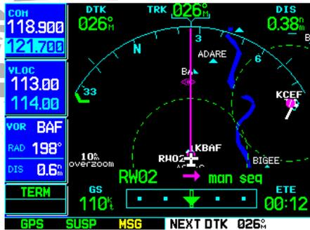
STEP 2: As you depart the airfield, "NEXT DTK 026°" appears in the lower right corner and "SUSP" appears above the **OBS** key. Indicated distance increases and is FROM the waypoint fix.
