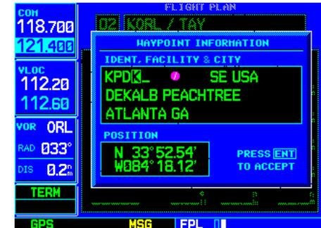
Use the **small** and **large right knobs** to enter the identifier of each flight plan waypoint.
