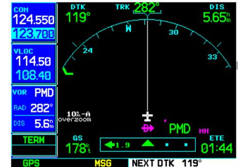
STEP 4 & 5: Upon reaching the desired altitude, press **OBS** to return to automatic leg sequencing. An alert message ("NEXT DTK 133°") appears guiding you to the inbound course.
