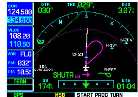
STEP 7: “START PROC TRN” appears in the lower right corner of the screen to remind you to initiate the procedure turn.
