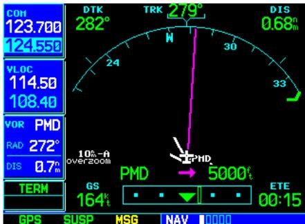
STEP 2: Within a few seconds of pressing **OBS** to start the missed approach, “SUSP” re-appears above the **OBS** key.
