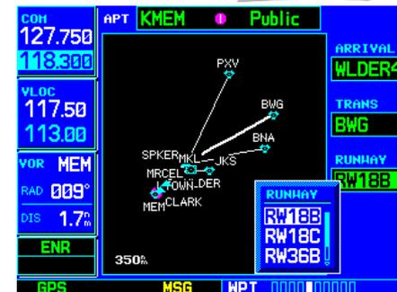
STEP 7: With the "RUNWAY" field highlighted, rotate the **small right knob** to select the desired runway. Many arrivals apply to all runways for a particular airport, as indicated by "ALL".
