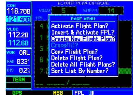
From the Flight Plan Catalog, press **MENU** to display the options menu and select “Create New Flight Plan?”.
