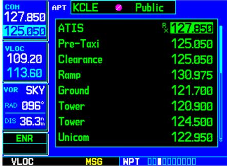
Listed communication frequencies include ATIS, clearance delivery, ground control, tower, unicom, approach and departure. The “RX” next to ATIS identifies it as a “receive only” frequency.
