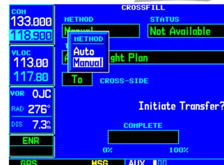
STEP 2: From the METHOD field, rotate the **small right knob** to select “Auto” or “Manual”. “Auto” automatically transfers direct-to or active flight plan selections between units.
