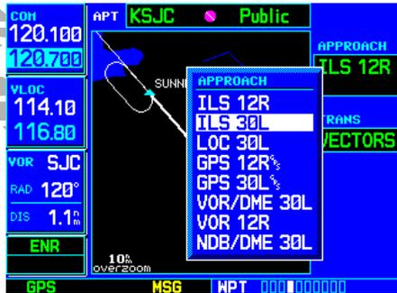
STEP 3 & 4: With the cursor on the “APPROACH” name field, rotate the **small right knob** to select the desired procedure and press **ENT**.
