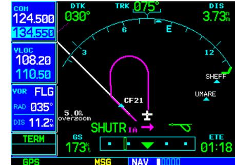
The GNS 530 can use its internal GPS receiver to guide you on the initial portion of an ILS approach. At this stage "GPS" is indicated above the **CDI** key.
