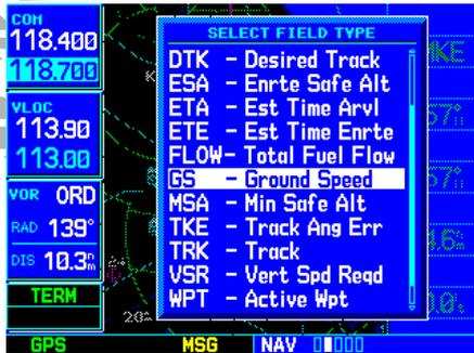
Once “Change Fields?” is selected, rotate the **large right knob** to highlight the data field you wish to change, then rotate the **small right knob** to select the type of data to display in that field.
