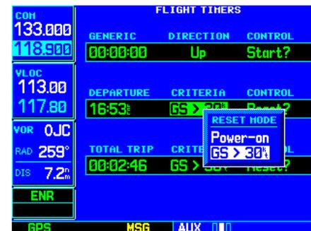
STEP 3 (bottom): The GNS 530 can be configured to record the departure time when the unit is powered on or when your ground speed exceeds 30 knots.
