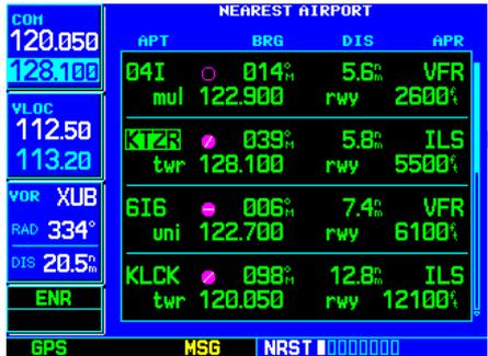
STEP 3 & 4: Highlight the identifier of the desired airport and press **ENT** to display the database information — beginning with location and fuel.
