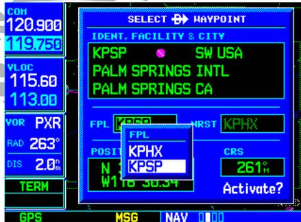
The flight plan (FPL) field allows you to select any active flight plan waypoint as your current destination waypoint.
