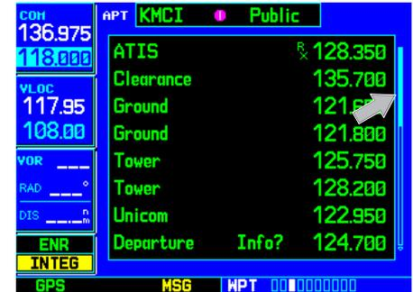
Whenever the GNS 530 is displaying a list of information that is too long for the display screen, a scroll bar appears along the right-hand side of the display. The scroll bar graphically indicates the number of additional items available within the selected category.
