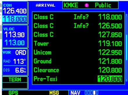
The scroll bar along the right-hand side of the page indicates the length of the NAVCOM frequency list and what portion of the list is currently being displayed.
