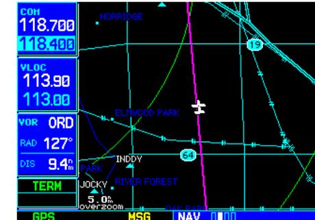
The Map Page is the second of four Nav pages (five if equipped with weather and/or traffic systems). The map scale is depicted in the lower left corner and adjusted with the **RNG** key.
