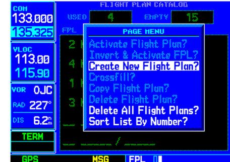
To create a new flight plan, select “Create New Flight Plan?” from the Flight Plan Catalog Options.
