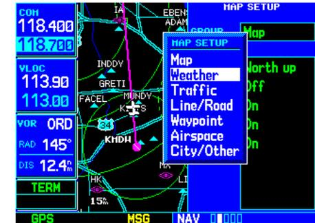
\* Weather and Traffic settings are only available when the GNS 530 installation includes connection to traffic and/or weather information sources. See 400/500 Series Display Interfaces Pilot's Guide Addendum.
