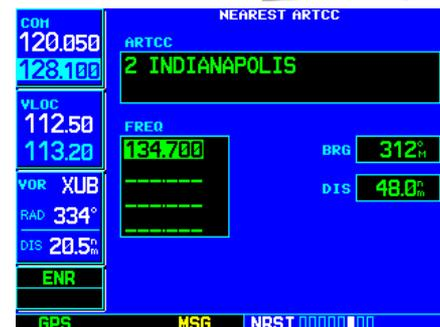
STEP 3 & 4: Rotate the **small right knob** to select the desired center, then rotate the **large right knob** to highlight the desired frequency.
