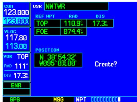
STEP 3 & 4: To enter a different position, highlight the position field and use the **small** and **large right knobs** to enter the new position coordinates.
