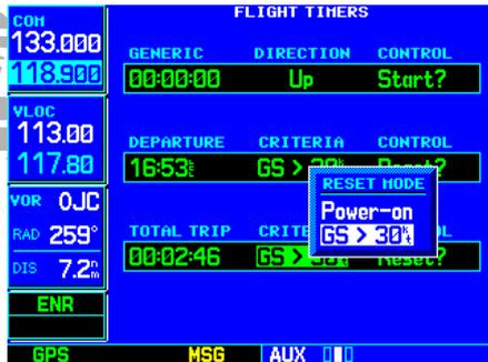
STEP 3 (top): Rotate the **small right knob** to select when the trip timer resets: each time the GNS 530 is powered on or when ground speed exceeds 30 knots.
