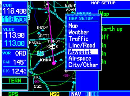
To select a map setup group, rotate the **small right knob**. Rotate the **large right knob** to highlight the desired setting within the group.
