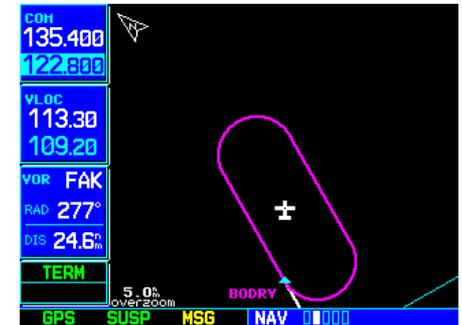
*STEP 10:* When crossing the IAF, “SUSP” appears above the **OBS** key to alert you that automatic waypoint sequencing is temporarily suspended.
