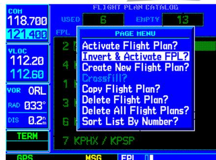
“Activate Flight Plan?” selects the highlighted flight plan and uses it for navigation guidance. “Invert & Activate FPL?” reverses the order of waypoints in the flight plan, then selects it for navigation guidance.
