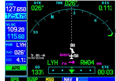
STEP 13: As you cross the missed approach point, "SUSP" appears on-screen above the **OBS** key. Press the **OBS** key to provide navigation guidance to the missed approach holding point.
