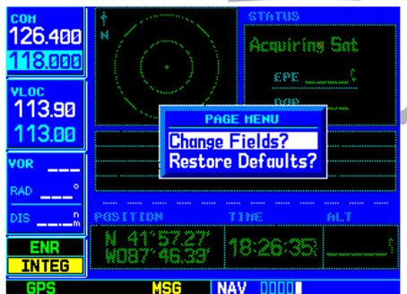
By default, current altitude (ALT) is displayed in the lower right corner of the page. This field is user selectable using the "Change Fields?" option.
