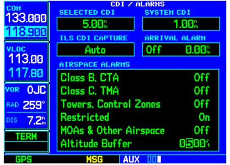
STEP 4: Use the **small and large right knobs** to enter the desired altitude buffer. This buffer distance is added to the floor/ceiling limits and provides an added margin of safety.
