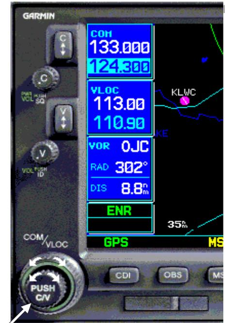
The **large** and **small left knobs** allow you to tune the desired COM or VLOC frequency.
