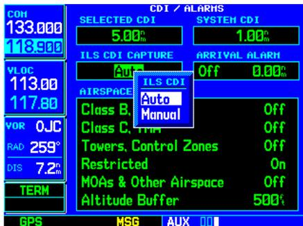
STEP 3 (middle): “Auto” ILS CDI Capture switches the CDI output from GPS to the VLOC receiver as you intercept the final approach course.
