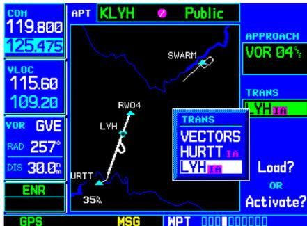
STEP 3: A second pop-up window displays available transitions. Highlight LYH VOR and press **ENT**. Finally, select “Load?” to add the approach to the active flight plan.
