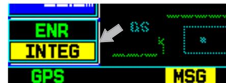
An "INTEG" annunciation at the bottom left corner of the screen indicates that satellite coverage is insufficient to pass built-in receiver autonomous integrity monitoring (RAIM) tests. When this occurs, the GPS receiver continues to provide navigation information, but should not be used for primary navigation guidance. Use the GNS 530's VLOC receiver or another suitable navigation source.
