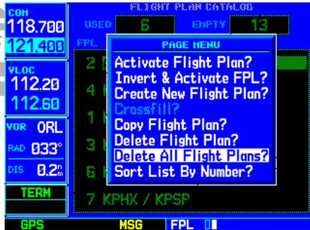
Select “Delete Flight Plan?” to remove the high-lighted flight plan from memory. “Delete All Flight Plans?” removes all flight plans from memory.
