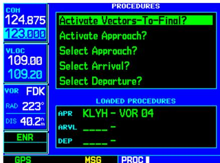
With the full approach “Loaded”, select “Activate Vectors-To-Final?” to provide navigation guidance along the final approach course segment only.
