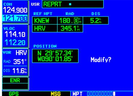
STEP 5: With the radial (RAD) field highlighted, use the **small** and **large right knobs** to enter a new radial from the reference waypoint.
