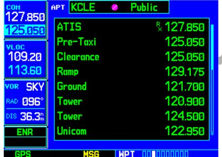
When the frequency list is too long to display on a single page, the scroll bar along the right-hand side of the list indicates the portion of the list that you are currently viewing (the shaded area) and the overall length of the list (indicated by the height of shaded and unshaded areas).
