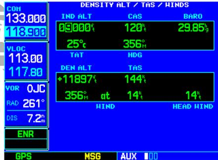
STEP 2: Use the **small** and **large right knobs** to enter the indicated altitude.
