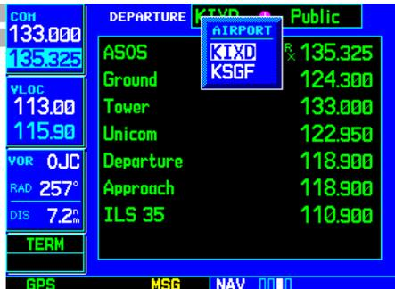
The Navigation/Communications (NAVCOM) Page provides a complete list of airport frequencies at your departure, en-route and arrival airports. To place a frequency from this list on standby, highlight the desired frequency and press **ENT**.
