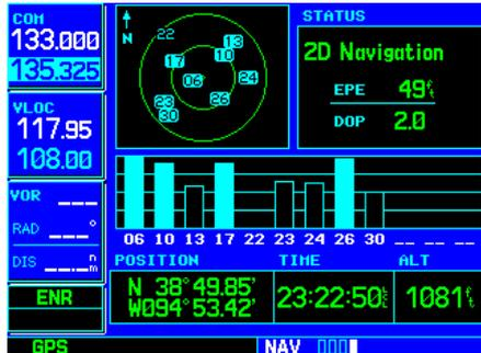
As satellites are received, the status changes to “2D Navigation” or “3D Navigation”. “3D Navigation” includes altitude, whereas “2D Navigation” is only the latitude/longitude position.
