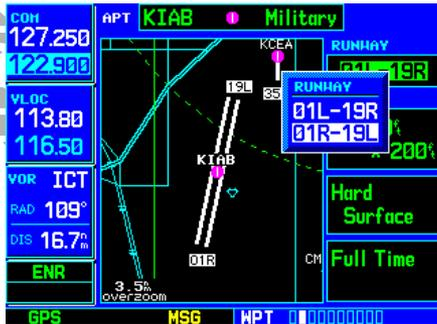
STEP 2 & 3 (top): Highlight the RUNWAY field and rotate the **small right knob** to display a listing of all runways at the selected airport.
