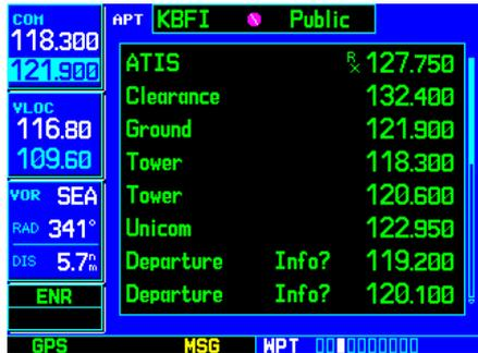
To view a different WPT page, the on-screen cursor should not be visible. (Press the **small right knob** to remove the cursor, if necessary.) Rotate the **small right knob** to select the desired WPT page.
