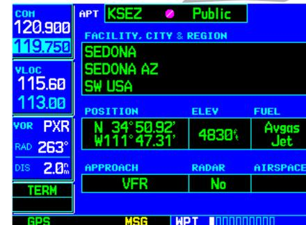
When a single waypoint is displayed on-screen, select it as your destination by pressing **direct-to**. When a list of waypoints is displayed, press the **small right knob** to display a cursor; highlight the desired waypoint, then press **direct-to**.
