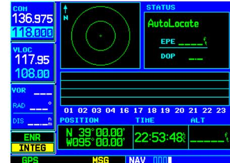
“AutoLocate” appears when the GNS 530 has orbital data, but last known position and/or time information are significantly different from current conditions.
