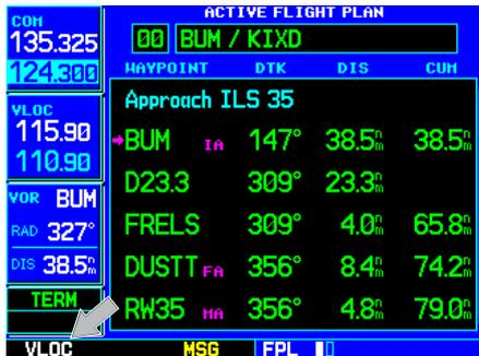
Press the **CDI** key to connect the external CDI (or HSI) to the VLOC receiver. Verify that “VLOC” appears directly above the **CDI** key.
