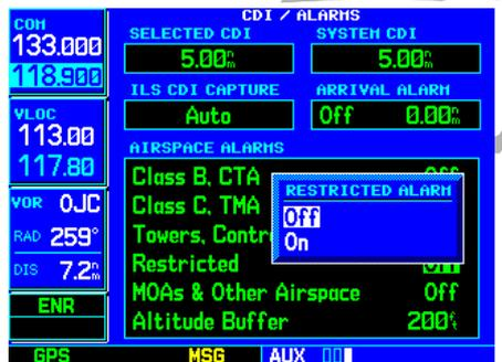
STEP 2 & 3: Rotate the **large right knob** to select the desired airspace type, then rotate the **small right knob** to select “On” or “Off”.
