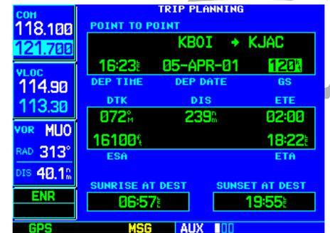
The Trip Planning Page calculates desired track, distance, estimated time en route, en-route safe altitude and estimated time of arrival for a specified direct-to, point-to-point or flight plan.
