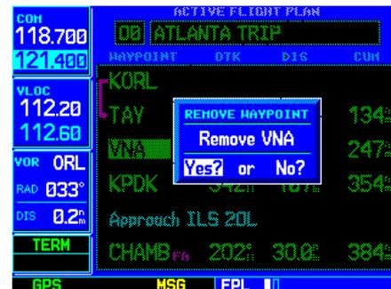
To remove an individual waypoint from the active flight plan, highlight the waypoint you wish to remove and press **CLR**.
