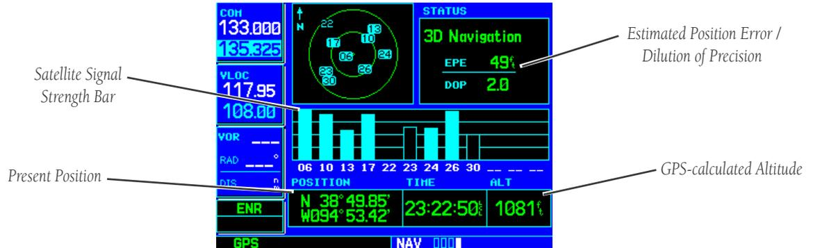
As the GPS receiver locks onto satellites, a signal strength bar appears for each satellite in view, with the appropriate satellite number (01-32) underneath each bar. The progress of satellite acquisition is shown in three stages:
