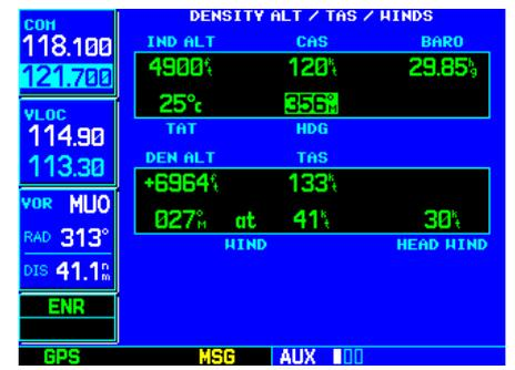
Select the “Density Alt / TAS / Winds” option to calculate density altitude, true airspeed and winds aloft.
