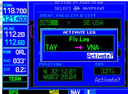
From the Active Flight Plan Page, use the **direct-to** key (press twice) to activate a highlighted route leg...
