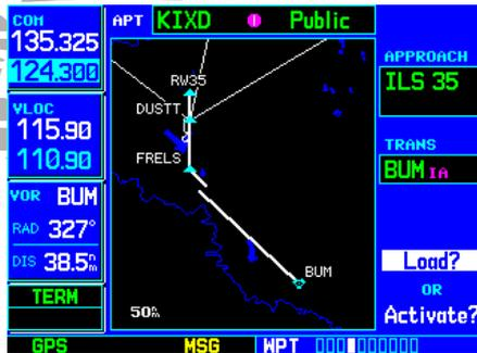
STEP 6 & 7: Select “Load?” or “Activate?” and press **ENT**. Verify that the navigation frequency is automatically placed on standby. To activate the frequency, press the **VLOC flip-flop** key.
