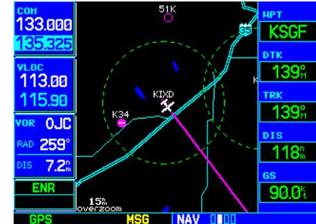
By adding data fields along the right-hand side, the Map Page can combine a moving map display and navigation data for complete situational awareness. Map setup pages are provided to add these data fields and to designate the maximum scale at which each map feature appears. These settings provide an automatic decluttering of the map (based upon your preferences) as you adjust the scale.
