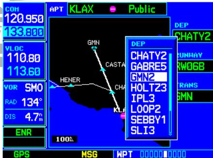
STEP 2 & 3: With the cursor on the “DEP” field, rotate the **small right knob** to display a list of available departure procedures.
