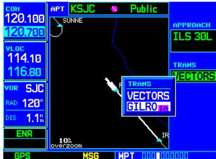
STEP 5: With the cursor on the “TRANS” field, rotate the **small right knob** to select the desired transition. Select “VECTORS” for guidance only along the final course segment of the approach.
