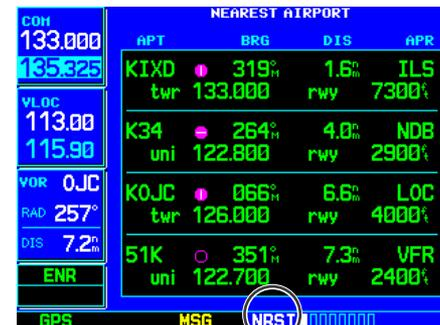
...then, rotate the **large right knob** to select the NRST page group, as indicated by "NRST" at the bottom of the screen. Rotate the **small right knob** to select the desired page within the group.
