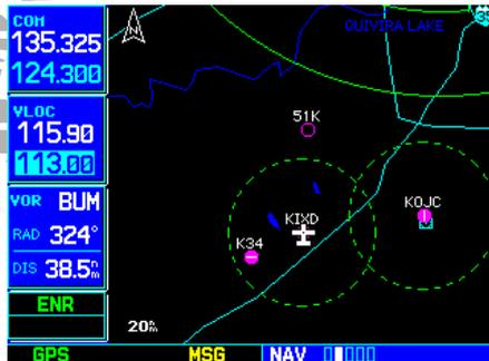
Press the **small left knob** to move the tuning cursor to the VLOC window. Rotate the **small left knob** to select the kilohertz portion of the frequency and the **large left knob** to select the megahertz portion.
