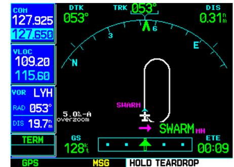
STEP 3: An alert message in the lower right hand corner recommends entry procedures for the holding pattern (e.g., "HOLD TEARDROP").
