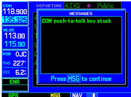
A “COM push-to-talk key stuck” message appears to warn you of a stuck microphone. Transmitting is disabled after 35 seconds of continuous broadcasting.
