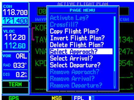
*Published instrument approaches can be selected and used from the Active Flight Plan Options, or by pressing the **PROC** key. The “Select Approach?” option appears in both places.*
