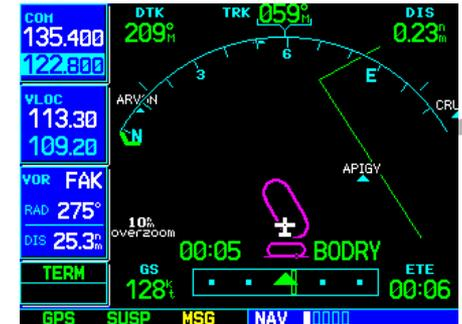
*STEP 9:* While flying the holding pattern, a timer appears on the Default NAV Page. Use the timer to fly the one minute outbound portion of the pattern.
