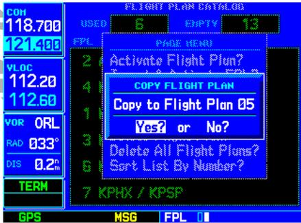
Use the “Copy Flight Plan?” option to save a copy of a flight plan to another memory location. This is useful for saving the active flight plan, or to save a stored flight plan before editing.
