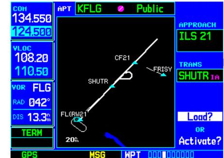
When an ILS approach is first selected, the ILS frequency is automatically placed in the standby VLOC frequency field. Press the **VLOC flip-flop key** to use this frequency.
