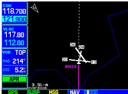
STEP 10: As you cross the MAP, “SUSP” appears above the **OBS** key, indicating that the automatic waypoint sequencing is suspended.
