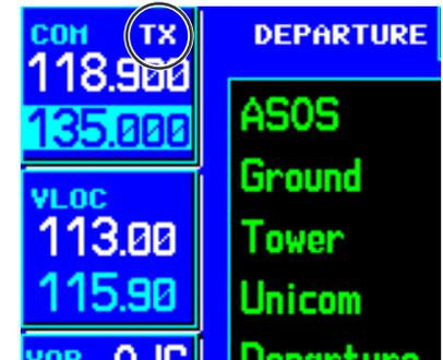
"TX" appears at the upper right corner of the COM window while transmitting.
