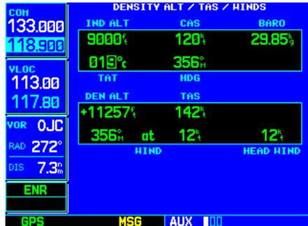
STEP 5: Use the **small** and **large right knobs** to enter the total air temperature (TAT). TAT is the temperature, including the heating effect of speed, read on an outside temperature gauge.
