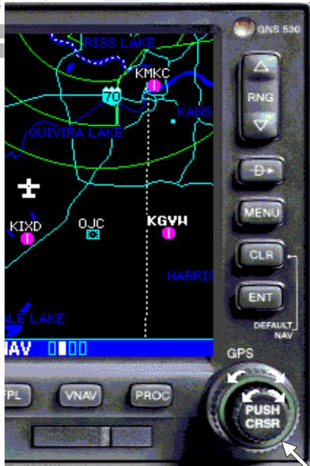
Data is entered using the **large and small right knobs**. Experiment with them to become efficient at entering data. This greatly reduces the amount of time spent operating the GNS 530 in flight.
