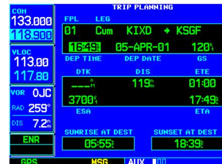
STEP 6: The current time and date are automatically offered for departure time and date. To accept either automatic selection, simply press **ENT** when the selection is highlighted.
