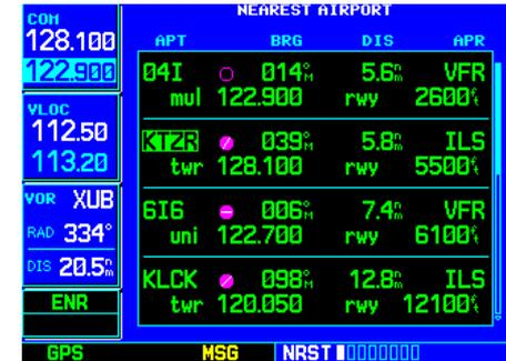
STEP 1 & 2 (bottom): You can select a direct-to destination directly from a NRST page (e.g. Nearest Airports) by highlighting the desired waypoint and pressing the **direct-to** key.
