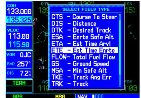
The **large right knob** is used to select the data field you wish to change. Then use the **small right knob** to display a list of data options and select the desired data item.
