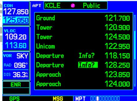
When "Info?" appears to the left of a displayed frequency, the frequency has usage restrictions.
