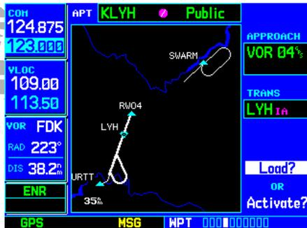
When an approach is “Loaded”, it is added to the end of the active flight plan. Prior to reaching the approach course, select “Activate Approach?” to begin navigation along the approach course.
