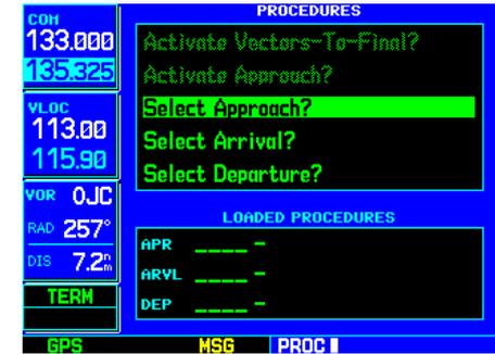
Press the **PROC** key to display the procedures page. Rotate the **large right knob** to select the desired option.
