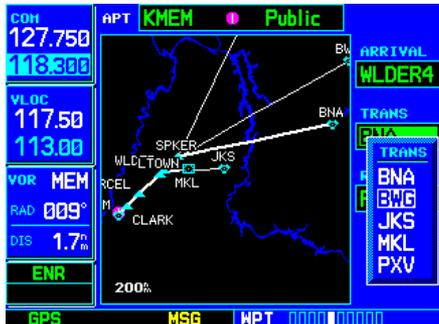
STEP 5: With the cursor on the “TRANS” field, rotate the **small right knob** to display a list of available transitions.
