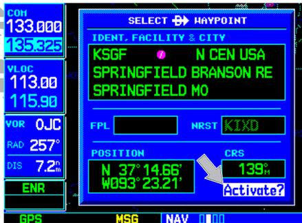
Confirm the selected direct-to destination by highlighting “Activate?” and pressing **ENT**.
