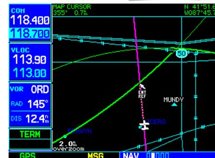
Once “Measure Dist?” is selected, place the on-screen pointer on the point you wish to measure FROM and press **ENT**.
