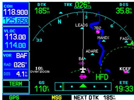
STEP 3 & 4: Once cleared to the next leg, press **OBS**. An alert appears indicating the desired track and the unit sequences to the next waypoint.
