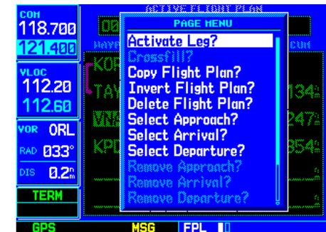
"Activate Leg?" selects the highlighted flight plan leg as the leg currently in use for navigation guidance (even if it isn't the closest leg).
