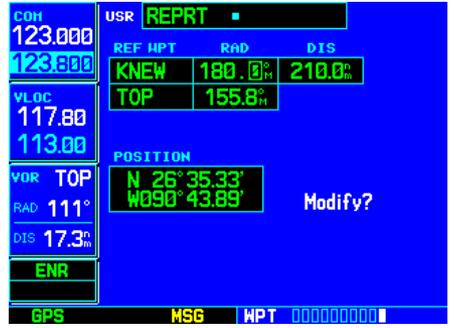
STEP 5: Use the **small** and **large right knobs** to enter the radial from the reference waypoint to the new user waypoint.
