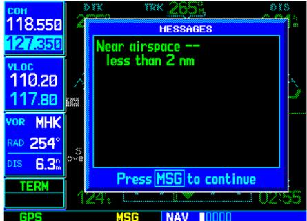
“Near airspace less than 2nm” indicates that you are within two nautical miles of an airspace, but are NOT projected to enter the airspace.
