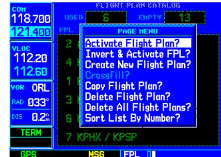
“Activate Flight Plan?” selects the highlighted flight plan for navigation guidance. “Invert & Activate FPL?” reverses the sequence of the highlighted flight plan, then activates it for navigation guidance.
