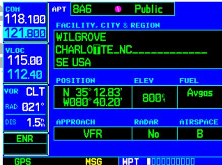
When selecting a waypoint by facility name or city, you can scroll through duplicate entries by continuing to rotate the **small right knob**.
