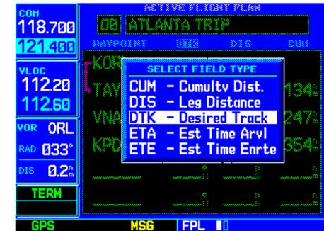
Change the displayed data using the "Change Fields?" option. Highlight the data field you wish to change and rotate the small right knob to display available data types.
