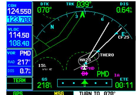
STEP 1: As the distance to the IAF approaches zero, the waypoint alert is replaced by a turn advisory ("TURN TO 070°"). Initiate a standard rate turn to this course heading.
