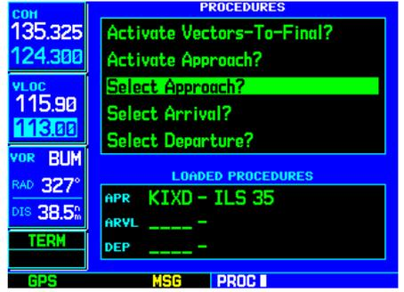
STEP 2 & 3 (bottom): When a VOR or localizer-based approach is “Loaded” or “Activated”, the frequency is automatically placed in the standby field of the VLOC window.
