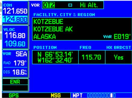
To display information for a VOR, highlight the identifier field. Then use the **small** and **large right knobs** to enter the VOR's identifier.
