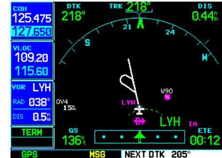
STEP 3: As you approach the IAF, the "NEXT DTK 205°" waypoint alert appears in the lower right corner. Prepare to turn to this heading.
