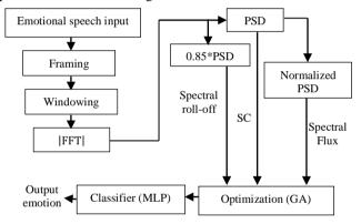
Fig. 1: Block diagram of the proposed emotion recognition system
