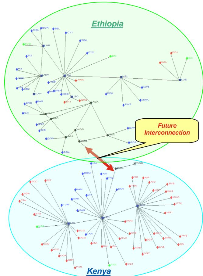
Fig. 3. Topology of the interconnected System Ethiopia – Kenya in GTMax Tool
