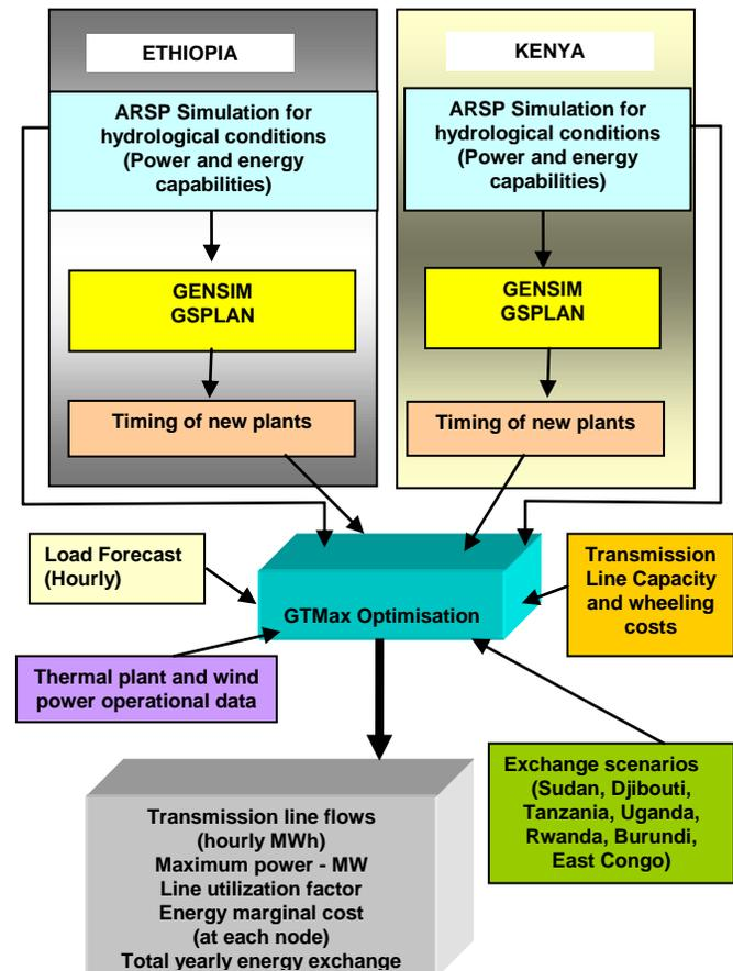
Fig. 2. Generation and Transmission Optimization using GTMax Tool
