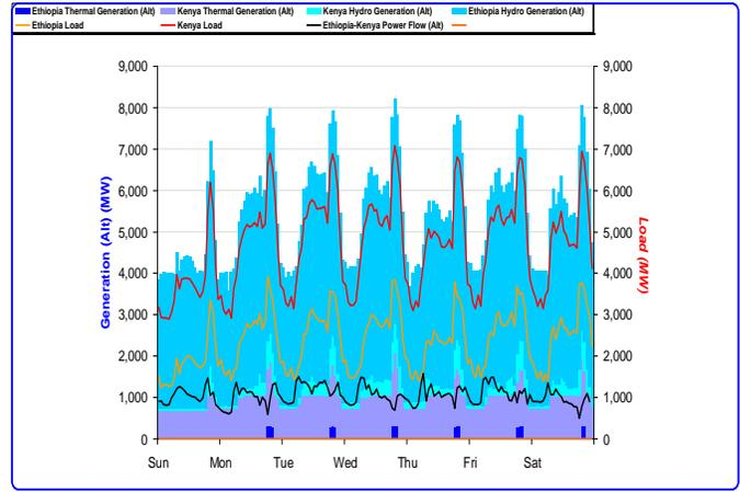
Fig. 7. GTMax simulation results for year 2023 (blue hydro generation, violet thermal generation, red load in Kenya, orange load in Ethiopia, black power flow on the interconnecting line)
