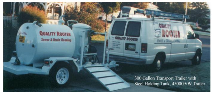
300 Gallon Transport Trailer with Steel Holding Tank, 4500GVW Trailer
