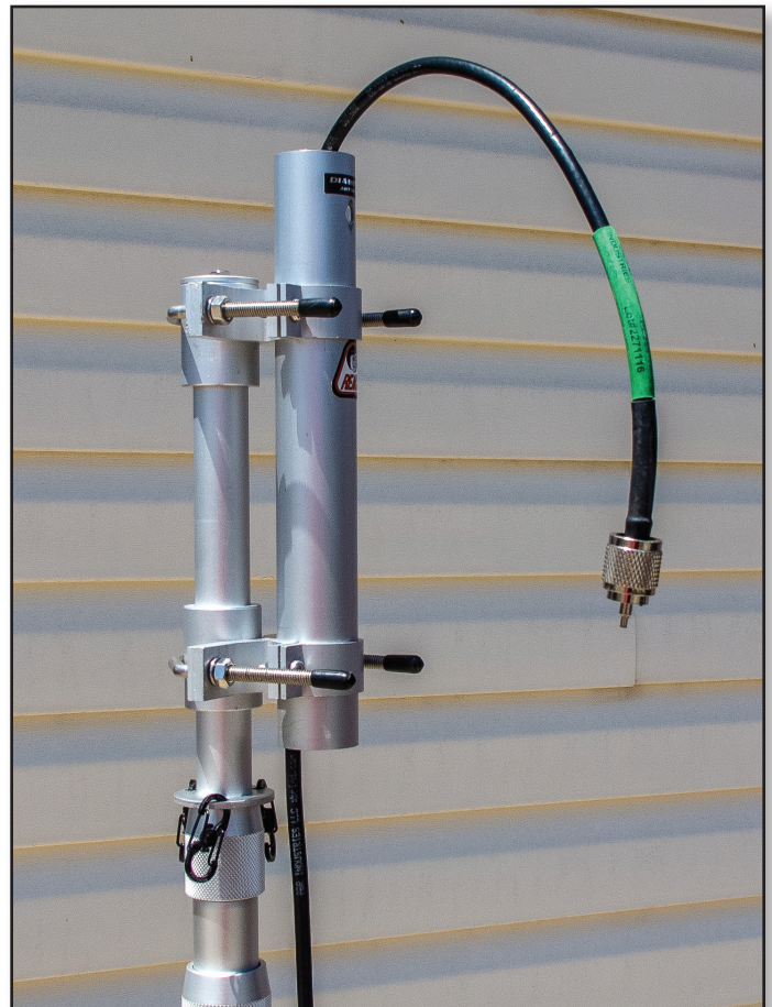
15. Coax threaded up through antenna support bracket.
