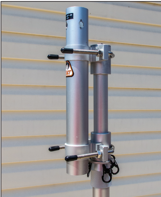
13. Antenna support bracket installed on mast.
