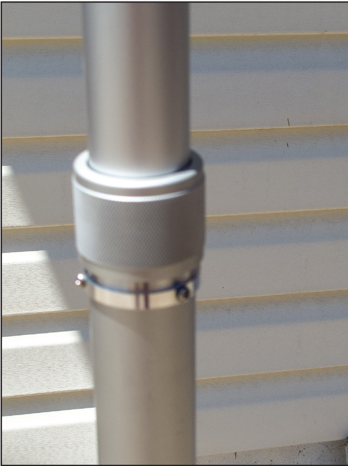
12. Knurled nut on tripod with mast inserted
