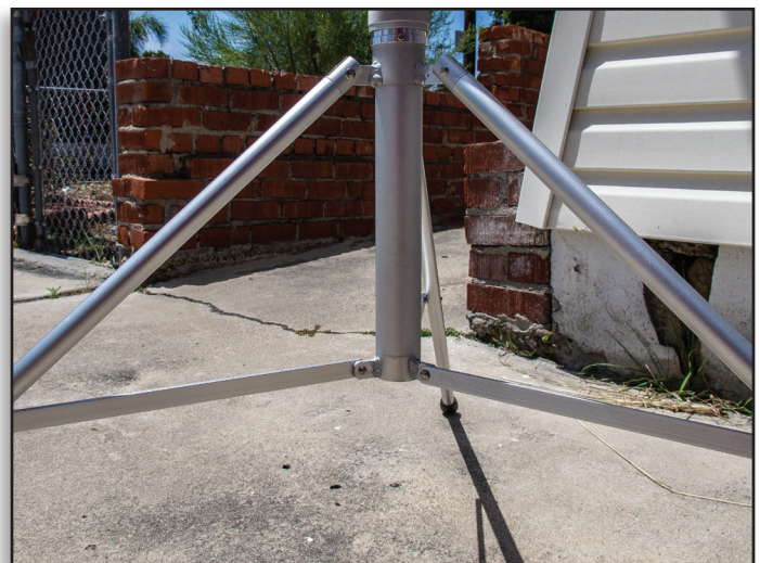
11. Tripod close-up. Note position of leg braces.
