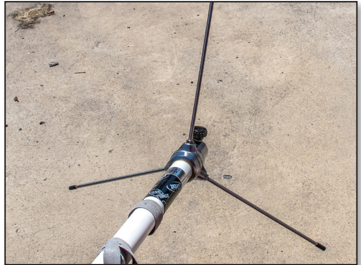
14. Radials attached to antenna.
