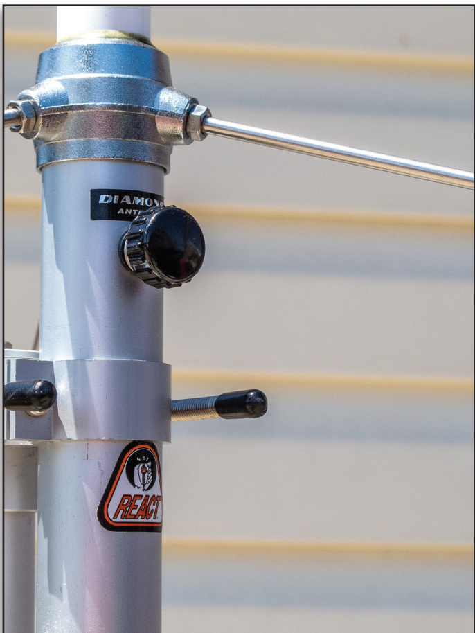
17. Close-up of knurled nut securing antenna to support.
