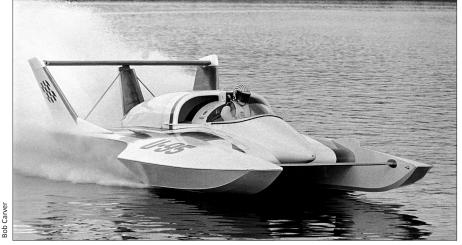
Chuck Lyford was the project manager for the U-95, the first turbine-powered unlimited hydroplane to compete in a race. Powered by a pair of Lycoming T-53s, the boat was owned by Jim Clapp, designed by Ron Jones, and driven by Leif Borgersen. The U-95 tested in September 1973, but Clapp died the following winter. His widow, Pamela, then campaigned the boat in 1974, until it sank during that year's Gold Cup race in Seattle. She and Chuck Lyford were married in 1991.
