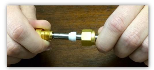
3. Slide the nut along with the PTFE ferrule up the shaft and connect to the cap by screwing the 2 pieces together trapping the ferrule in between as shown in the picture below. Hand tighten the compression cap and then use wrenches  $(9/16'' \& \frac{1}{2}'')$  to tighten another  $\frac{1}{4}$  turn. Gloves Recommended when handling tubes
