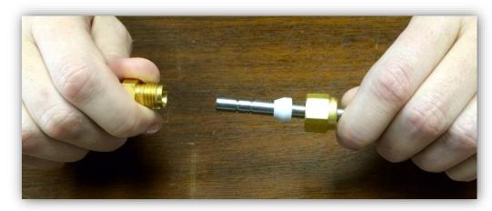
2. Place the top part of the cap onto the tube so that the end of the tube rests as far inside the cap as possible as shown in the picture below.
