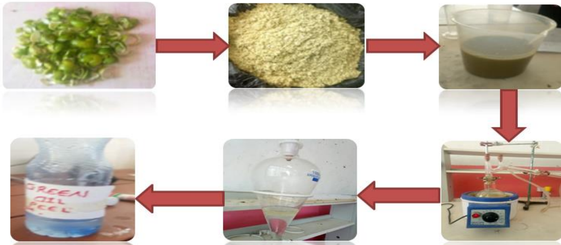
Figure 2. Extraction process of essential oils from green lemon peel
