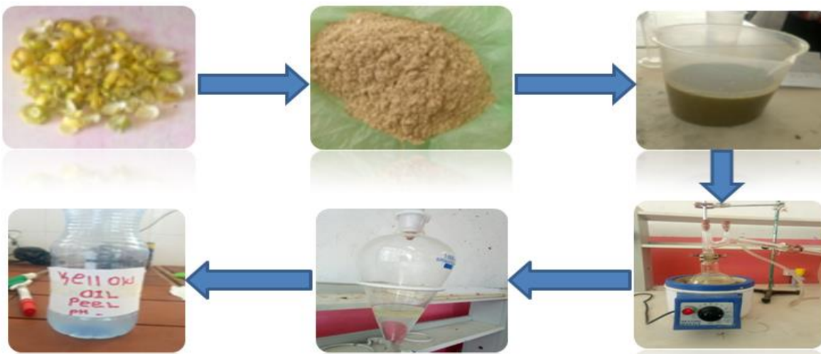
Figure 3. Extraction process of essential oils from orange lemon peel
