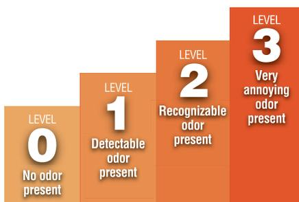
(measured as Dilutions-to-Threshold, or D/T). The laboratory dilution process simulates the dilution of the odor in the ambient air. There are specific rules and guidelines that cover who is qualified to be an odor assessor; for example, someone with chronic allergies would not be qualified. Assessors receive training in olfactory awareness, sniffing techniques, descriptor standards, and similar issues. Laboratory olfactometry is well-used by the food and fragrance industries.
