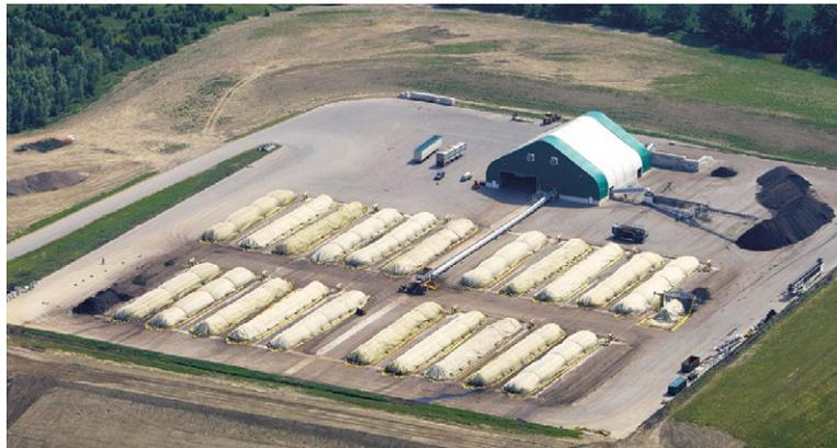
**The Region of Peel curing facility ran into a firestorm of odor complaints when it first opened using an open-air windrow system. Establishment of a public liaison committee and extensive outreach and education, plus installation of a GORE cover system, has yielded positive results.**
