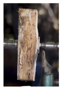
Start the lathe at slow speed, increase speed to confortable level without vibration (faster is better on intermittent cuts). Using bowl gouge with a pull cut start removing some of the bulk of the log and cut a tenon for your chuck. I continue shaping the bottom of bowl keeping tool rest close to log, (always turn lathe off when moving tool rest and then re-check that wings clear rest and banjo). As wood is removed and log becomes more balanced I continue to turn speed up, (faster is better).
