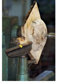
I do most of the shaping of the bottom of the bowl and bottom of the wing as it faces the tail stock between centers.
