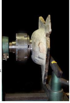
HINT: Tape can be used on tool rest to mark outermost swing of wing. (yellow tape photo above and left) to keep track of where to start or finish cuts.
