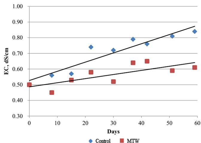
Fig. 4. EC accumulation over time - depth of 60 cm.
