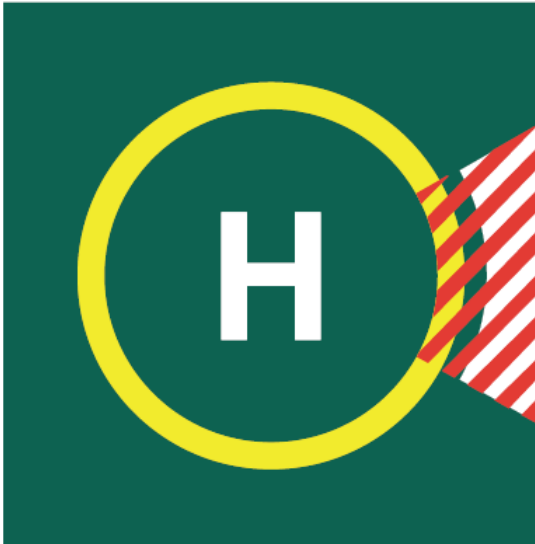
Figure 5 - Example of Prohibited Landing Heading Marking
