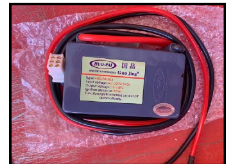
NEW IGNITER SYSTEM AS OF 2024
