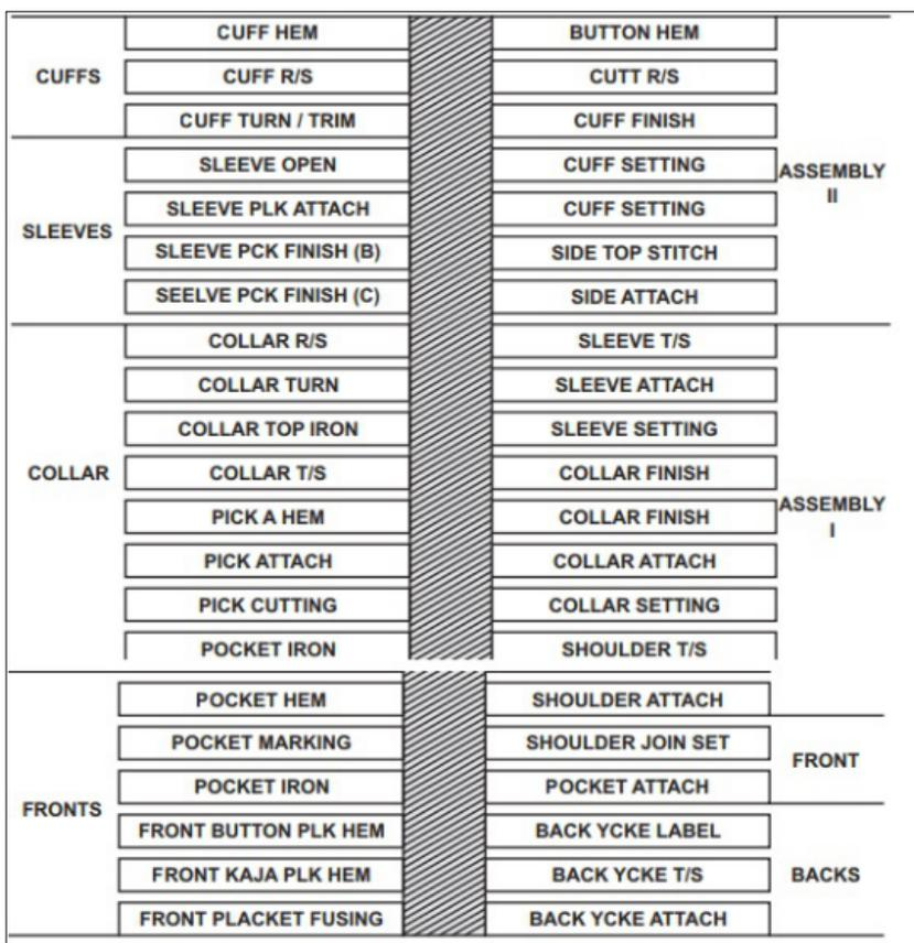
Figure 5 - Progressive Bundle system for shirt making
