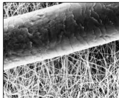
Fig. 6: Comparison of Nano fibre with conventional fibre
