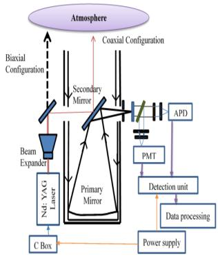
Figure 4. Schematic diagram of the lidar system developed
