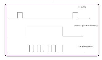
Figure 2. A timing diagram for Data Acquisition
