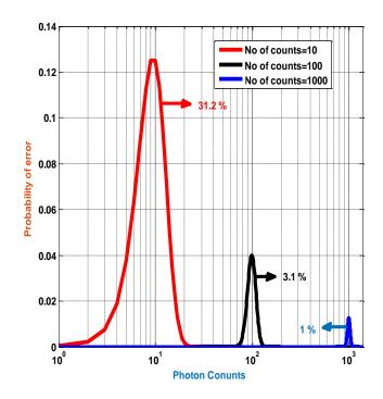
Figure 9 Photon counts vs Probability of error
