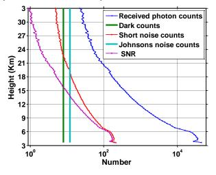
Figure 10 Estimation of SNR from the measured data
