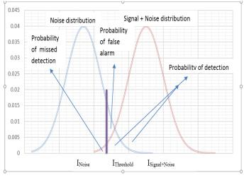
Figure 7 PDF of a Lidar return
